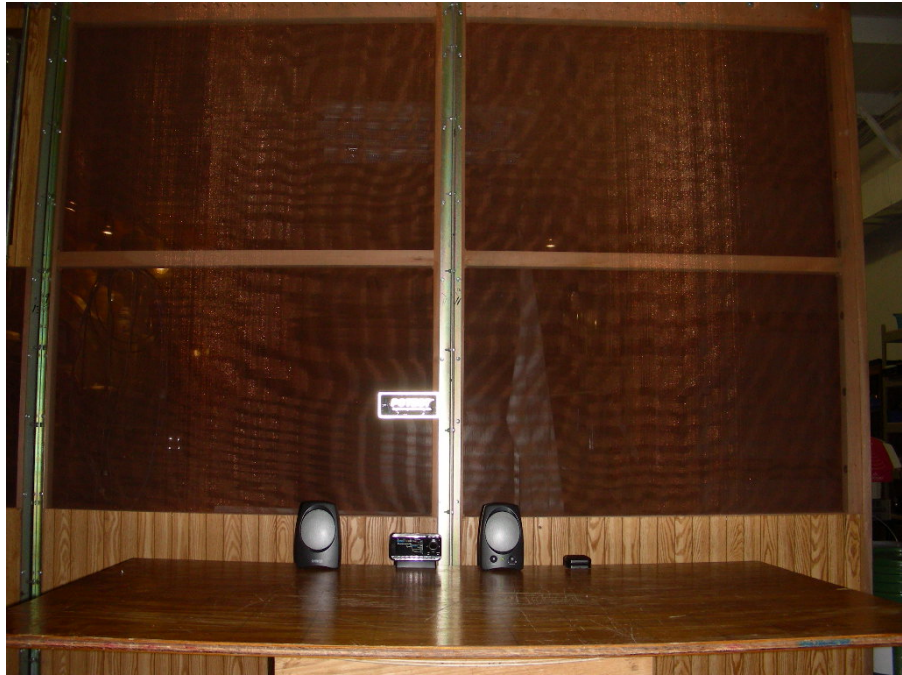
Test Configuration #1 – Conducted Emissions
