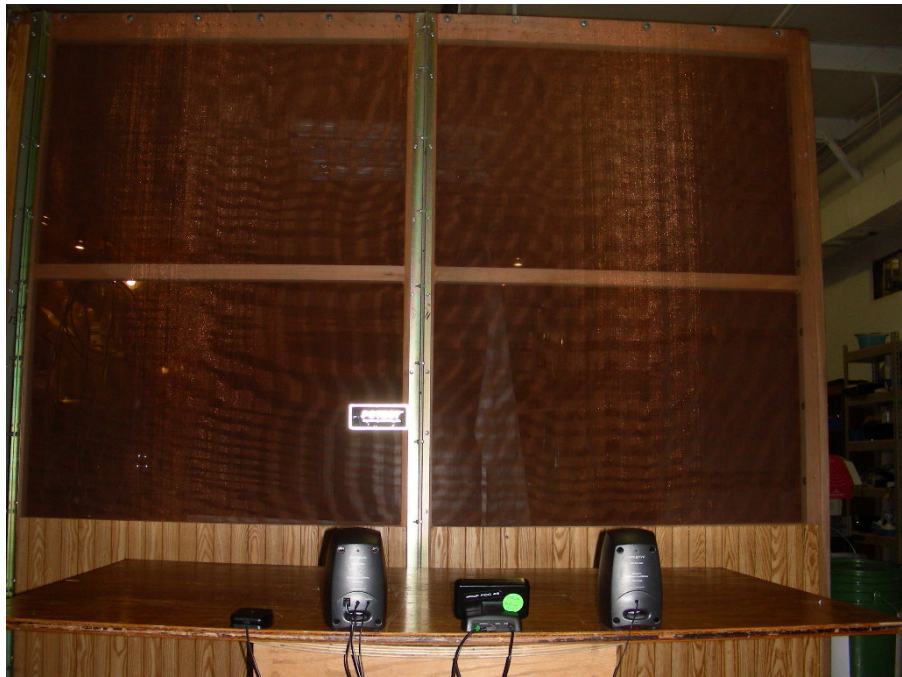
Test Configuration #1 – Conducted Emissions
