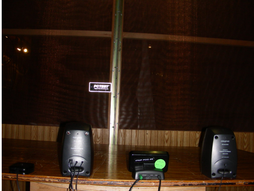
Test Configuration #1 – Conducted Emissions
