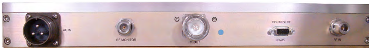
Figure 6-3 HPA Rear Panel Connectors
