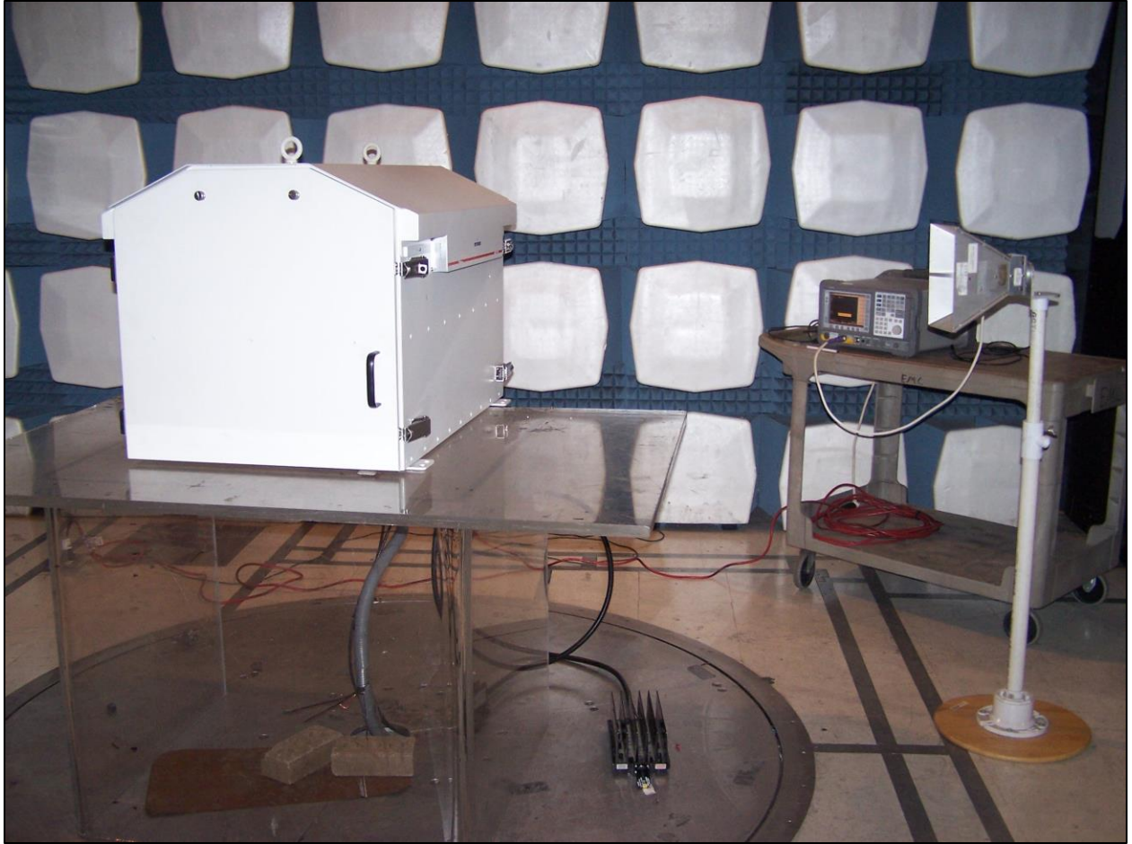
Photograph 5. Cabinet Radiated Emissions above 1 GHz
