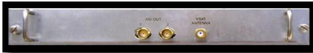
Figure 5, VSAT (L-Band) Receiver Panel
