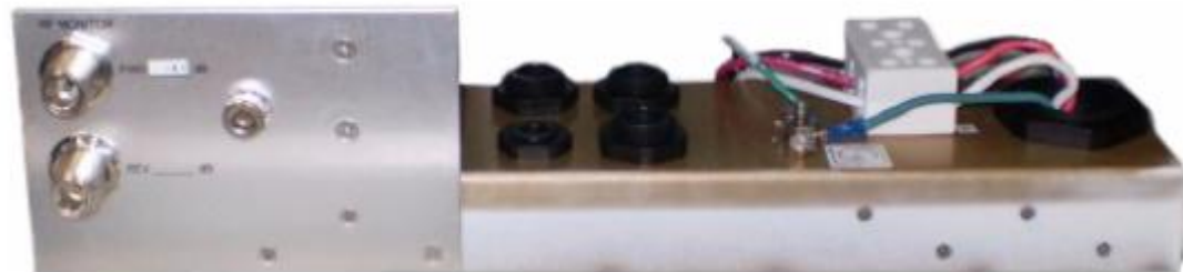
Figure 9, Junction Box Assembly Panel
