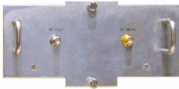
Figure 7, Up-Converter Module Panel
