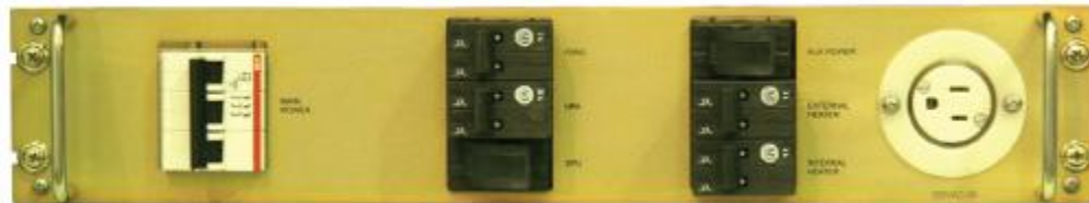
Figure 8, Power Distribution Unit Panel
