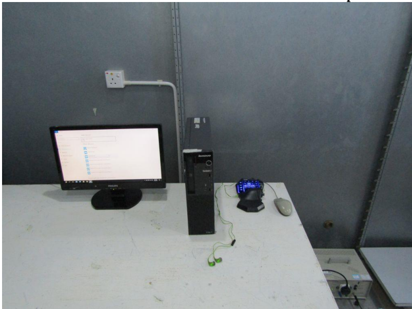
Measurement of Conducted Emission Test Set Up
