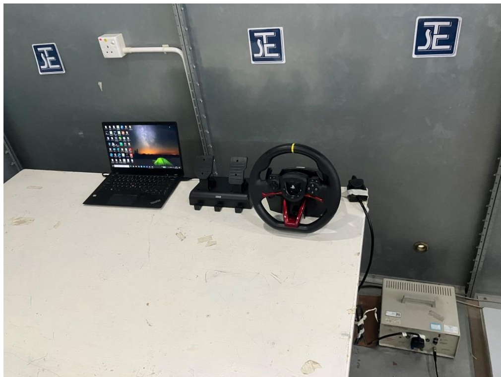
Measurement of Conducted Emission Test Set Up
