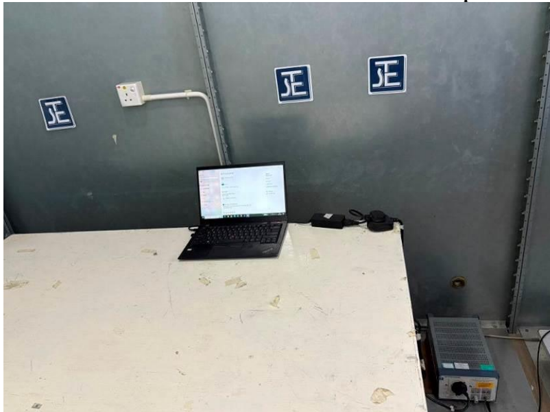
Measurement of Conducted Emission Test Set Up
