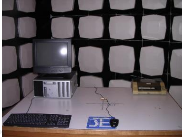
Measurement of Radiated Emission Test Set Up
