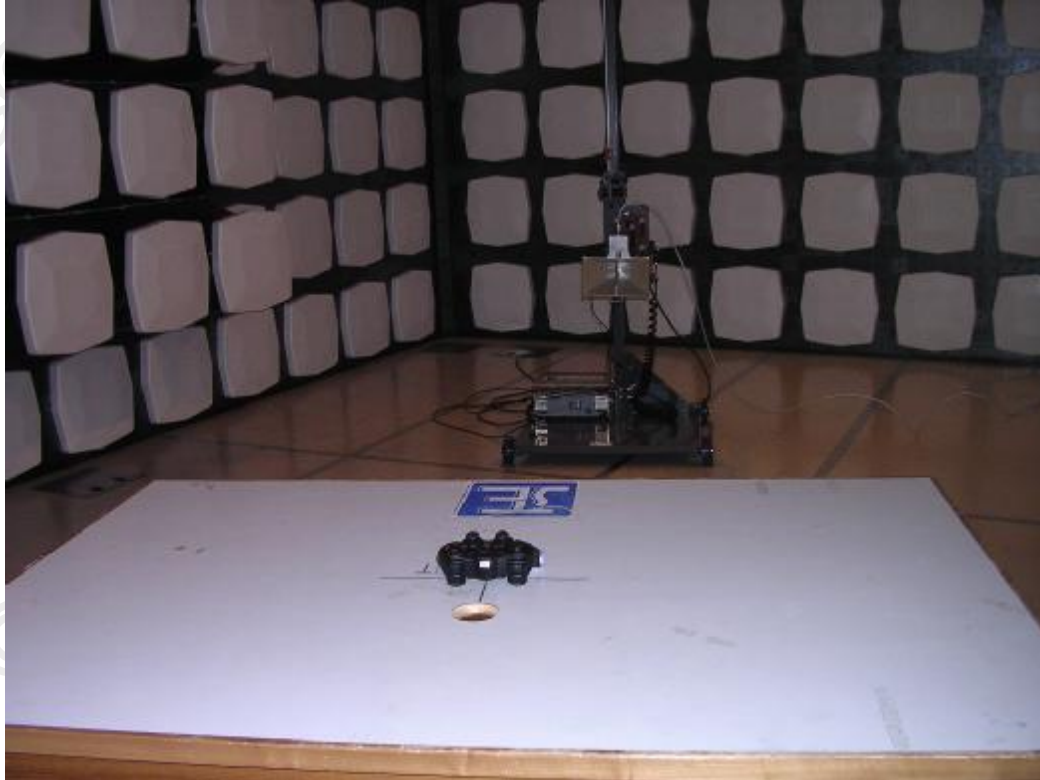
Measurement of Radiated Emission Test Set Up
