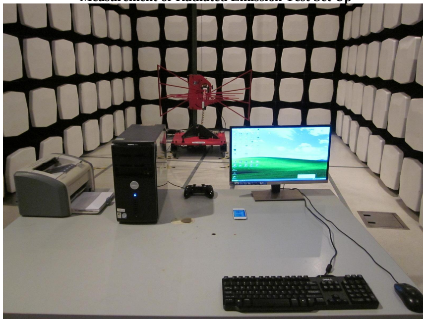
Measurement of Radiated Emission Test Set Up
