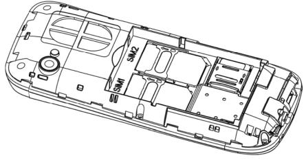
3.Put the SD card into card slot.
