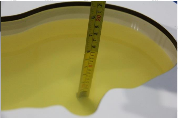
Liquid depth in the Head Phantom (1900MHz)
