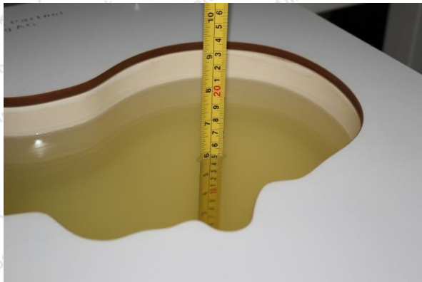
Liquid depth in the Head Phantom (1750MHz)
