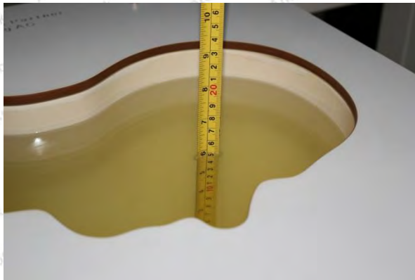
Liquid depth in the Head Phantom (1750MHz)
