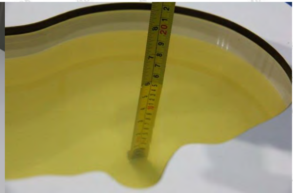
Liquid depth in the Head Phantom (1900MHz)
