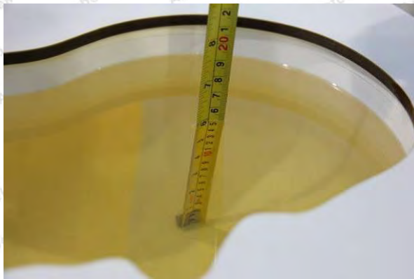
Liquid depth in the Head Phantom (750MHz)
