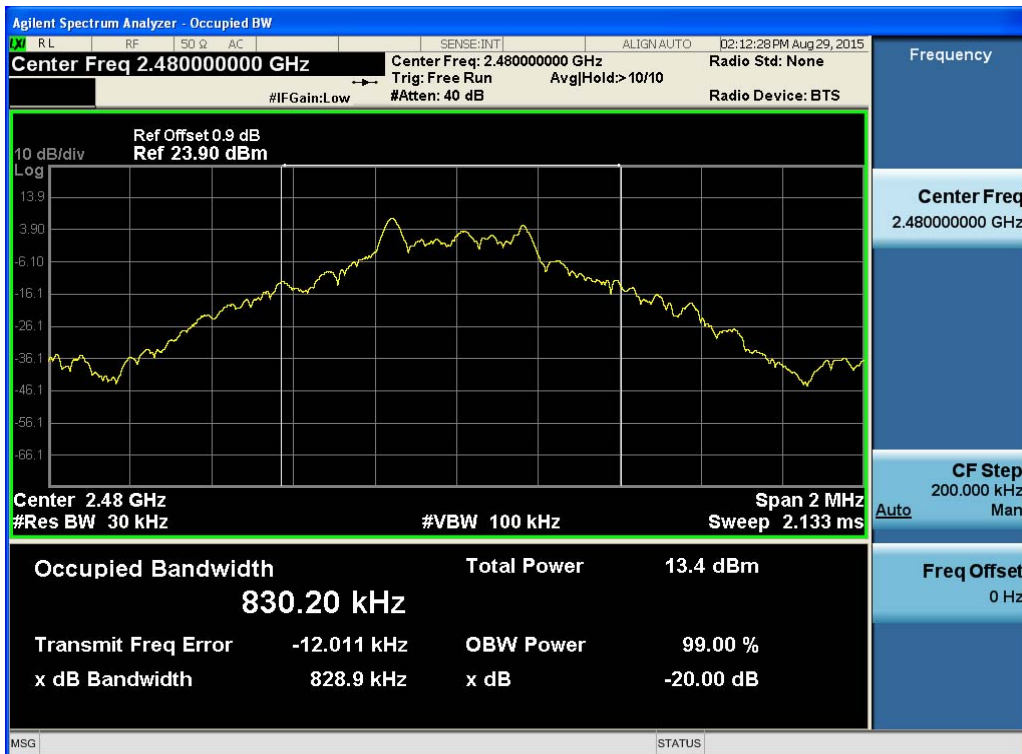
(Plot 4.4.1 C: Channel 78: 2480MHz @ GFSK)
