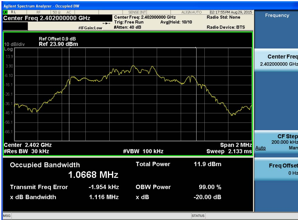
(Plot 4.4.2 A: Channel 00: 2402MHz @ 8DPSK)
