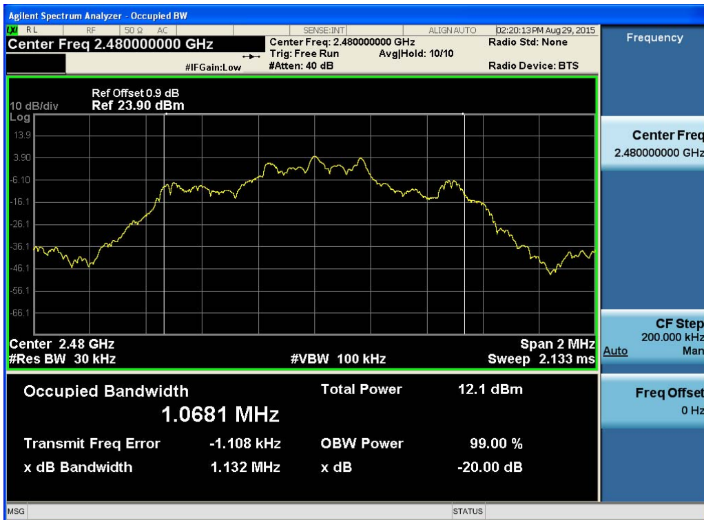
(Plot 4.4.2 C: Channel 78: 2480MHz @ 8DPSK)
