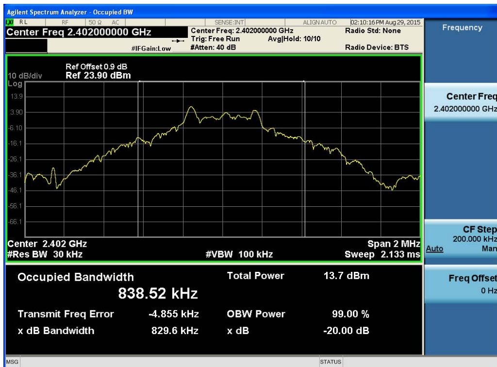
(Plot 4.4.1 A: Channel 00: 2402MHz @ GFSK)
