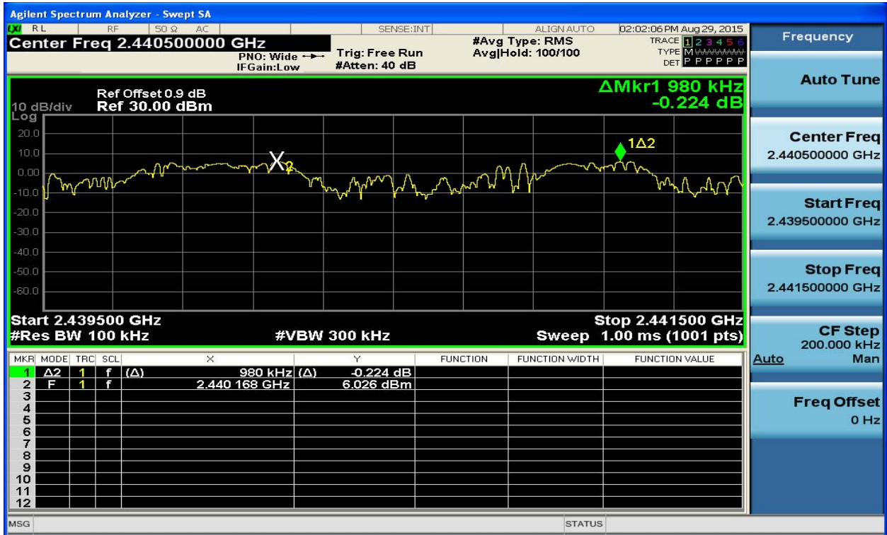
(Plot 4.6.2 A: Channel 39: 2441MHz @ 8DPSK)
