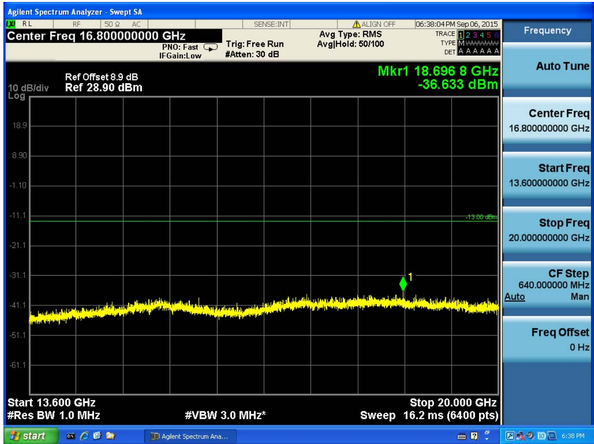
(Plot 4.5.3 C6: Channel 1513: 1752.6MHz @ Traffic WCDMA Band IV)
