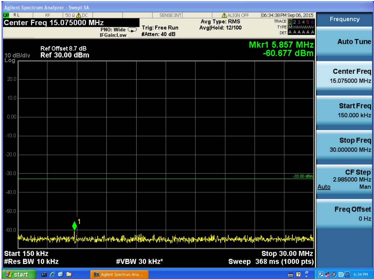
(Plot 4.5.3 A2: Channel 1312: 1712.4MHz @ Traffic WCDMA Band IV)
