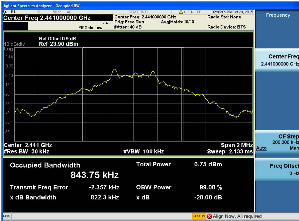
(Plot 4.4.1 B: Channel 39: 2441MHz @ GFSK)
