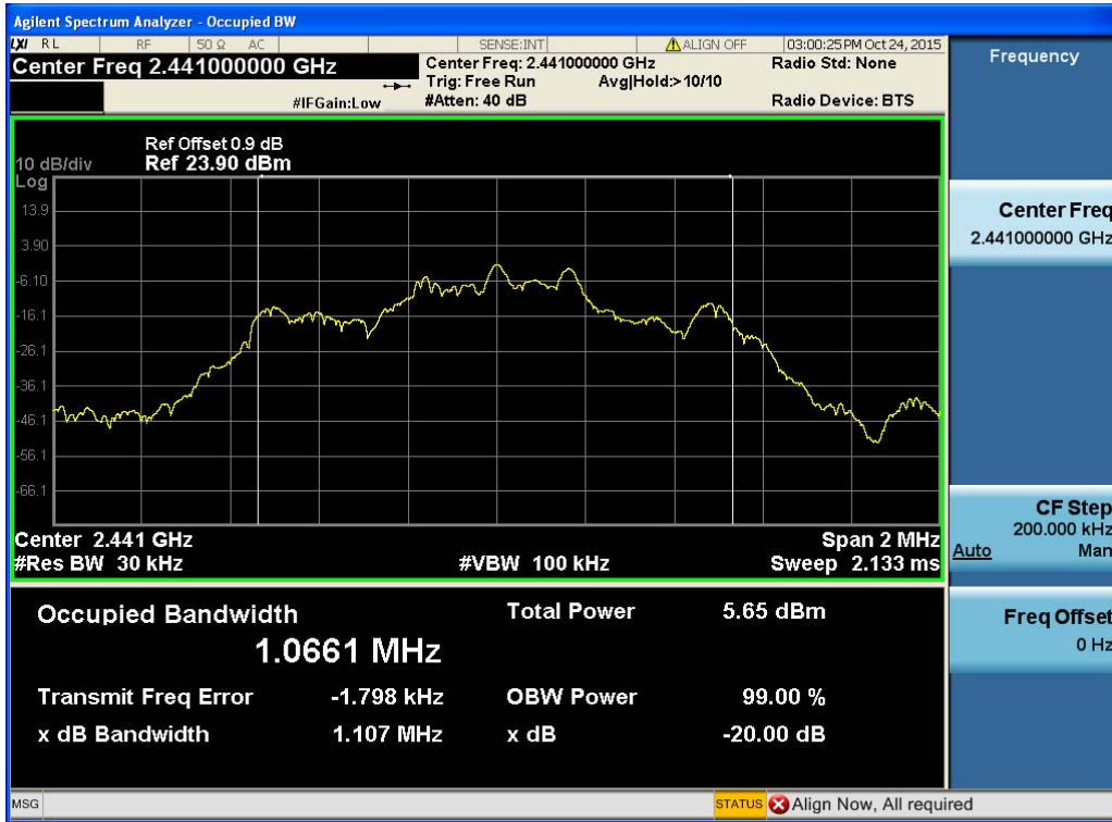
(Plot 4.4.2 B: Channel 39: 2441MHz @ 8DPSK)
