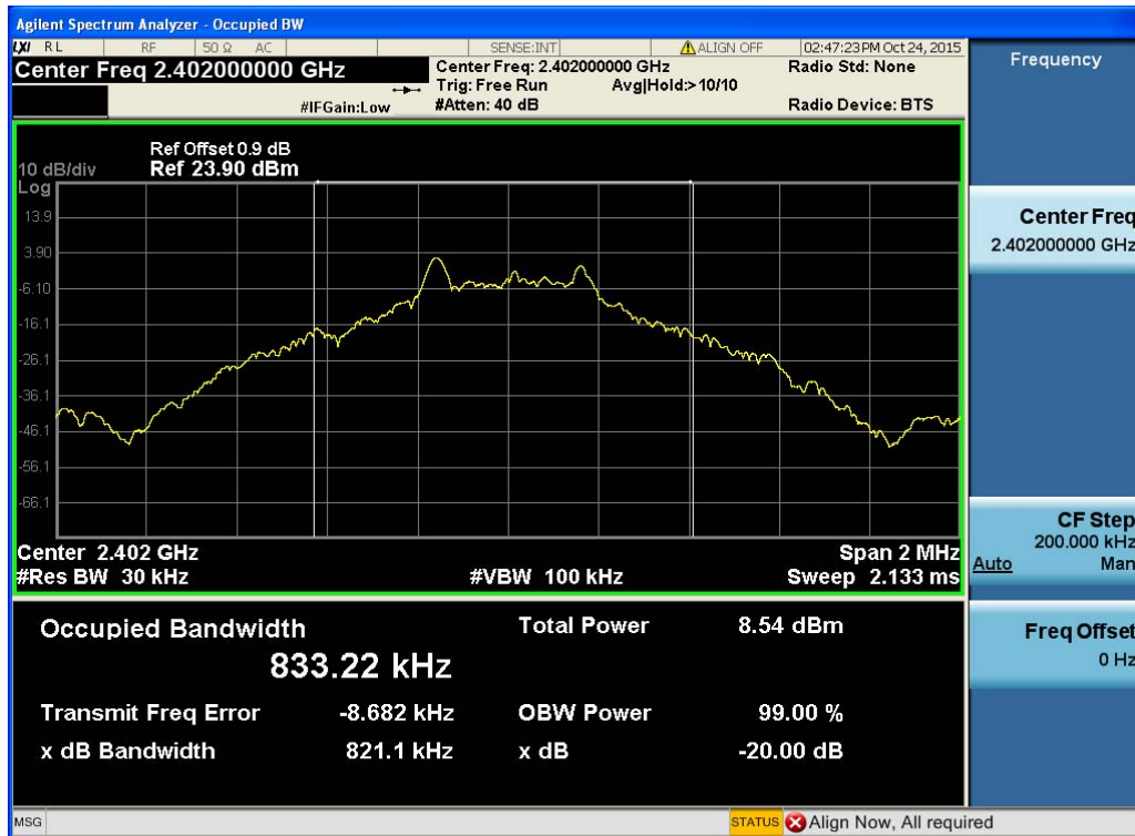
(Plot 4.4.1 A: Channel 00: 2402MHz @ GFSK)
