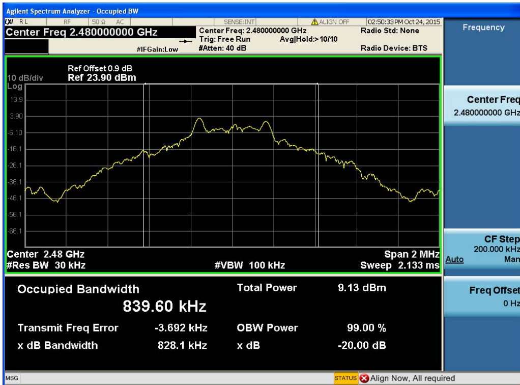
(Plot 4.4.1 C: Channel 78: 2480MHz @ GFSK)
