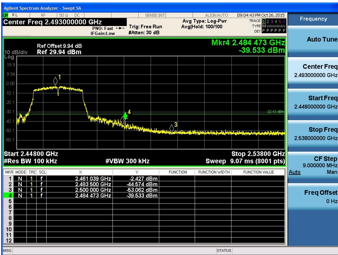
(Plot 4.5.2.2 B: Channel 11: 2462MHz @ 802.11 g)
