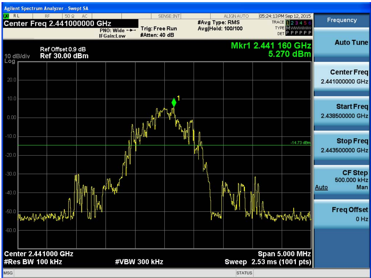
(Plot 4.9.2 B1: Channel 39: 2441MHz @ @ 8DPSK)
