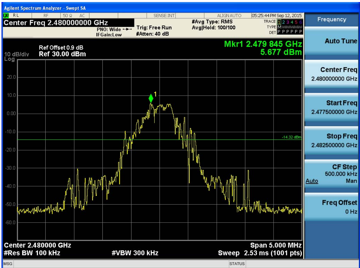
(Plot 4.9.2 C1: Channel 78: 2480MHz @ @ 8DPSK)
