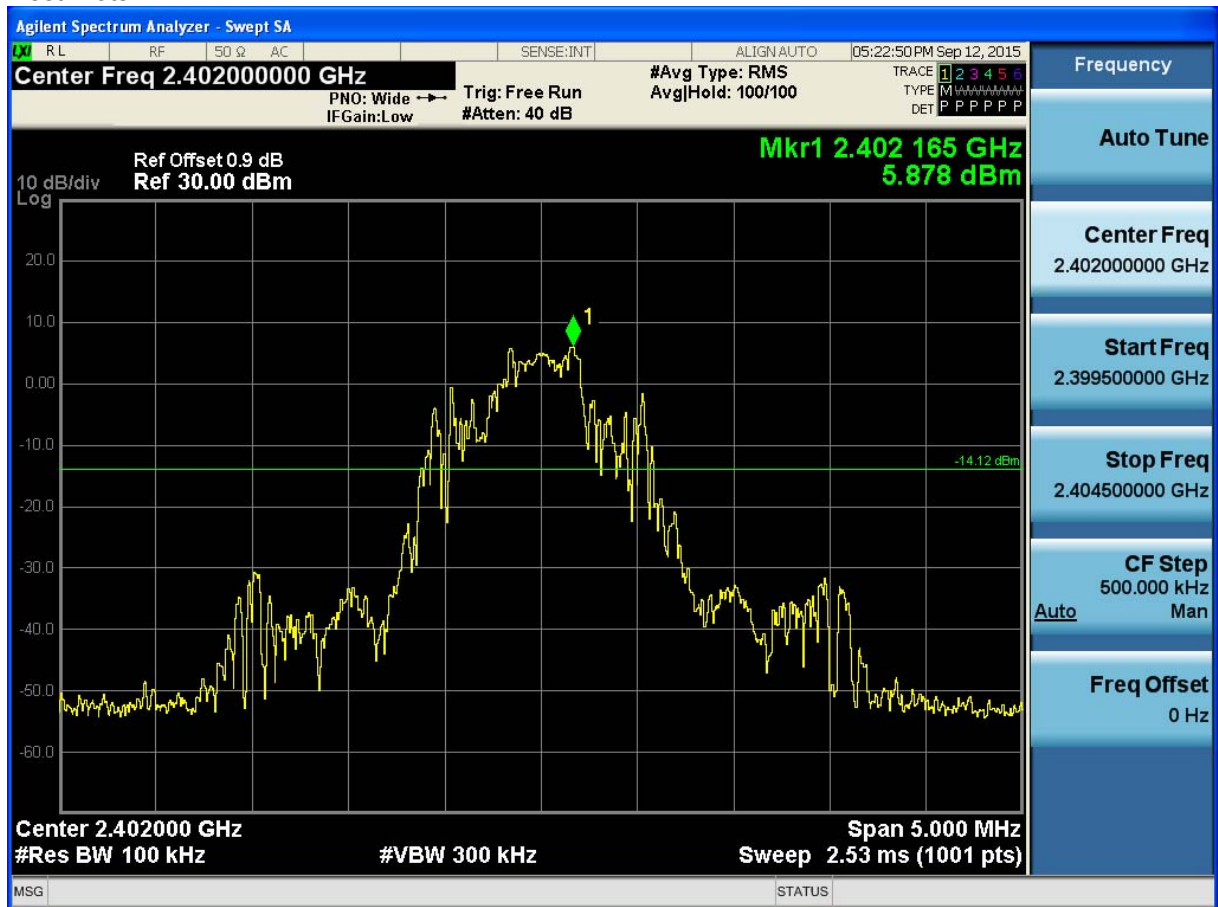
(Plot 4.9.2 A1: Channel 00: 2402MHz @ 8DPSK)
