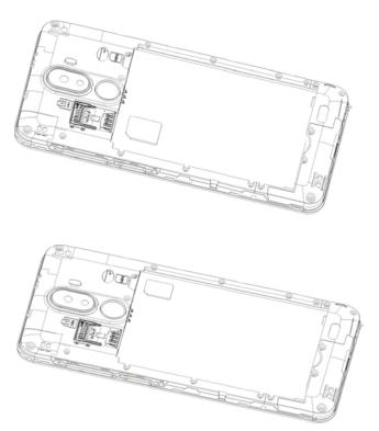
2. The SD card should be installed in the upper part of the SIM card 1.
