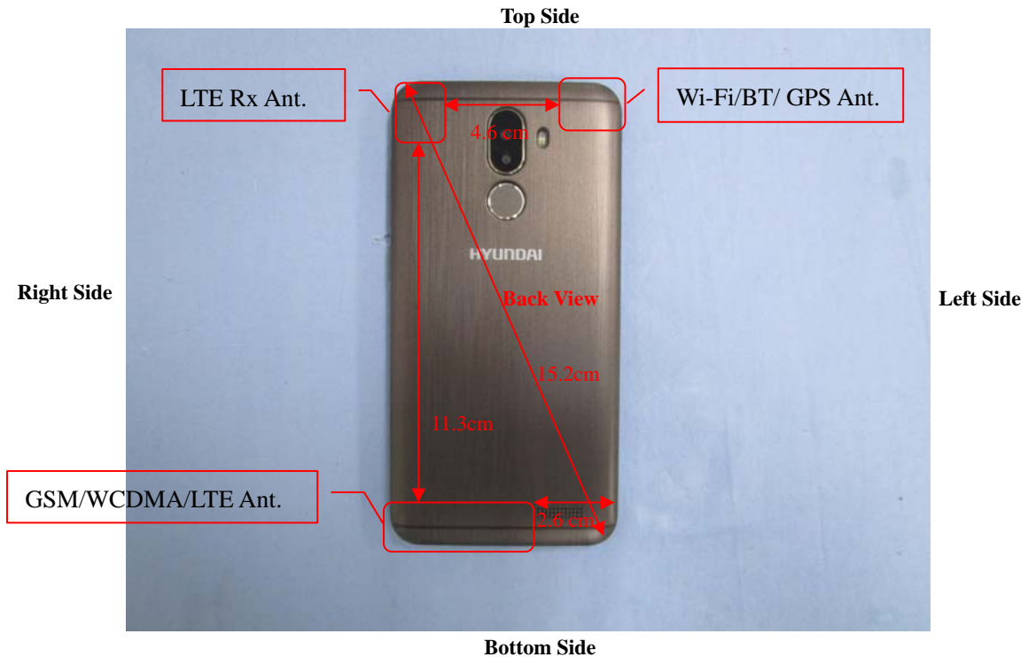
Block Diagram for EUT Antenna Position
