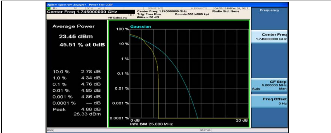
(Channel Bandwidth:20 MHz)_HCH_16QAM_1RB#99
