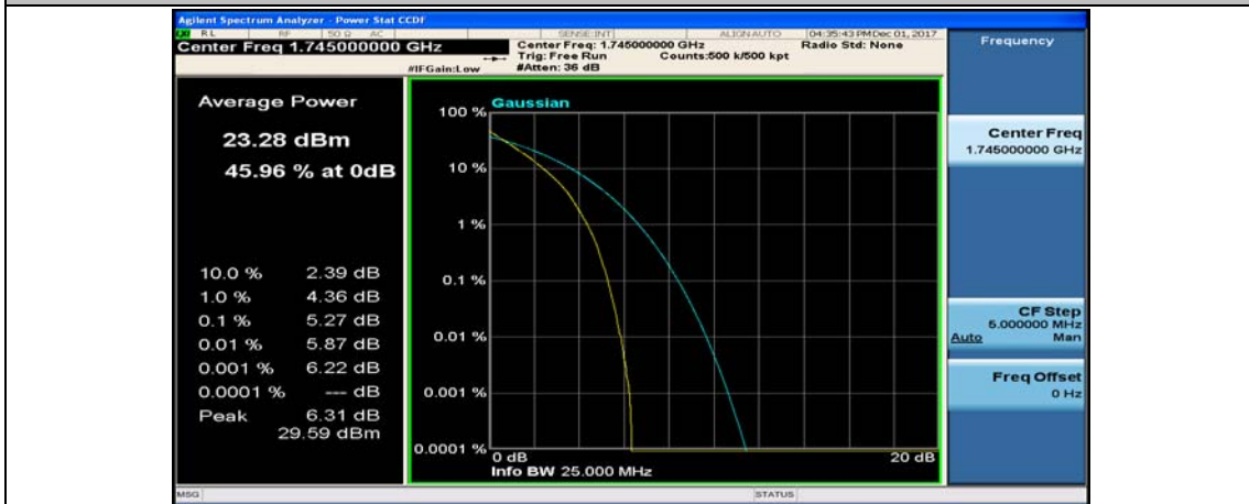
(Channel Bandwidth:20 MHz)_HCH_QPSK_100RB#0
