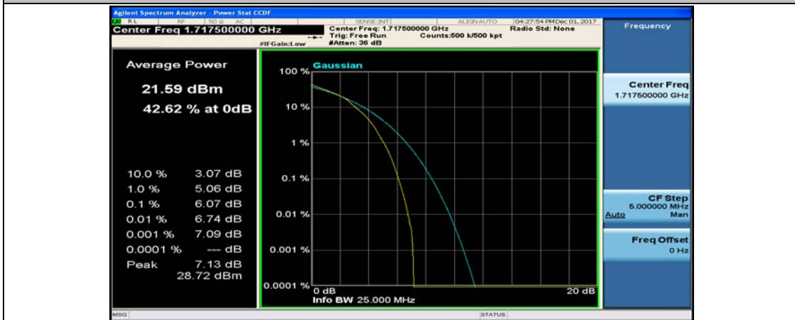
(Channel Bandwidth:15 MHz)_LCH_16QAM_75RB#0
