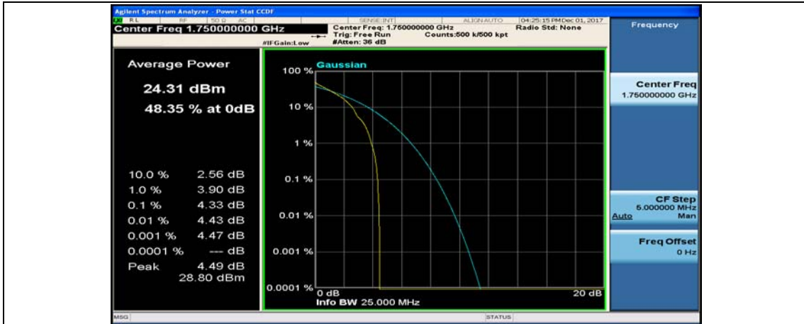
Channel Bandwidth: 10 MHz_HCH_QPSK_1RB#49
