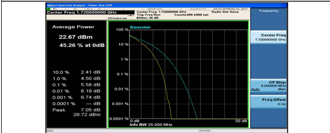
(Channel Bandwidth:20 MHz)_LCH_QPSK_100RB#0
