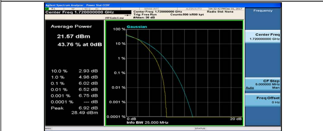
(Channel Bandwidth:20 MHz)_LCH_16QAM_50RB#50
