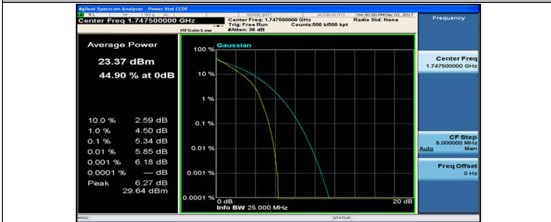
(Channel Bandwidth:15 MHz)_HCH_QPSK_75RB#0
