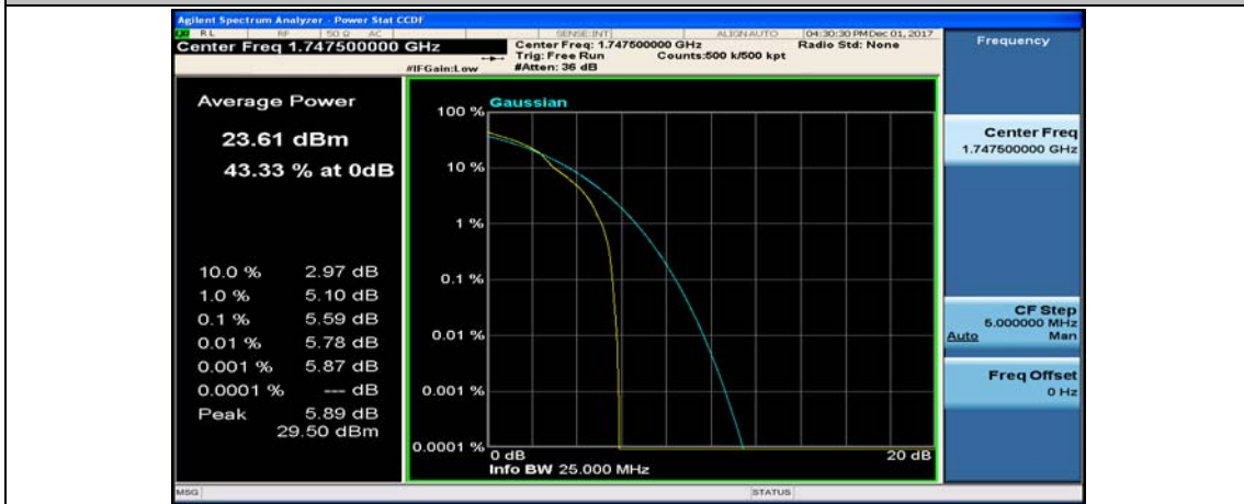
(Channel Bandwidth:15 MHz)_HCH_16QAM_37RB#0
