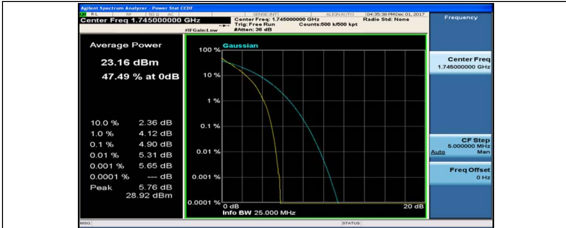
(Channel Bandwidth:20 MHz)_HCH_QPSK_50RB#50
