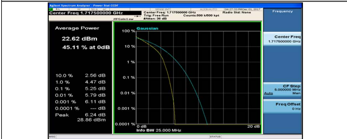
(Channel Bandwidth:15 MHz)_LCH_QPSK_75RB#0
