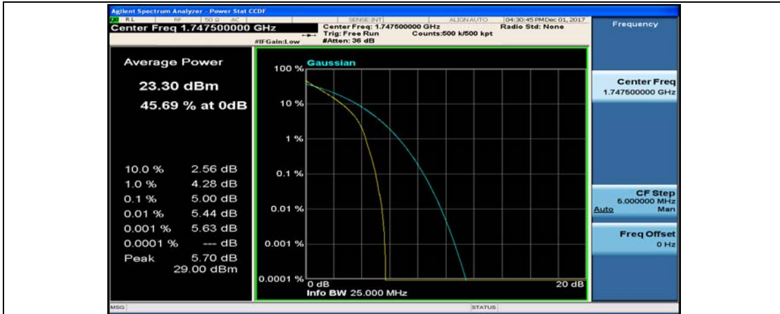
(Channel Bandwidth:15 MHz)_HCH_QPSK_37RB#38
