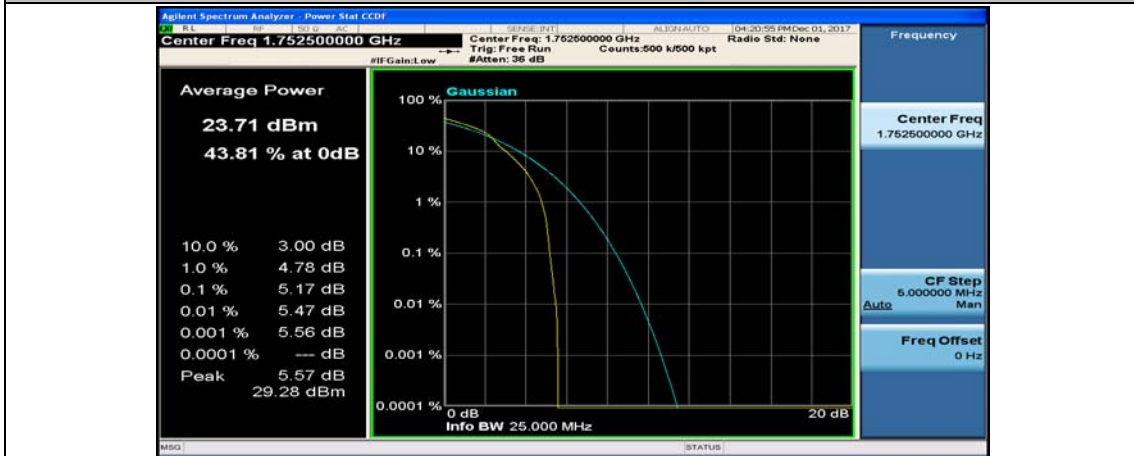
(Channel Bandwidth: 5 MHz)_HCH_16QAM_1RB#12
