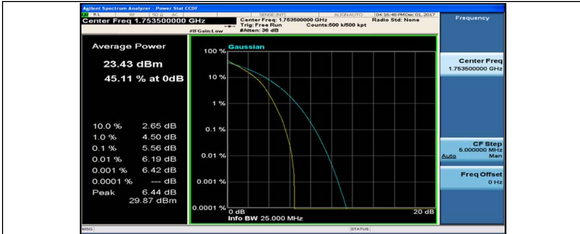
(Channel Bandwidth: 3 MHz)_HCH_QPSK_8RB#7
