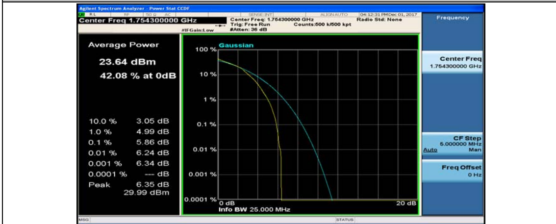
(Channel Bandwidth: 1.4 MHz)_HCH_16QAM_3RB#2
