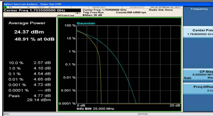
(Channel Bandwidth: 3 MHz)_HCH_QPSK_8RB#0
