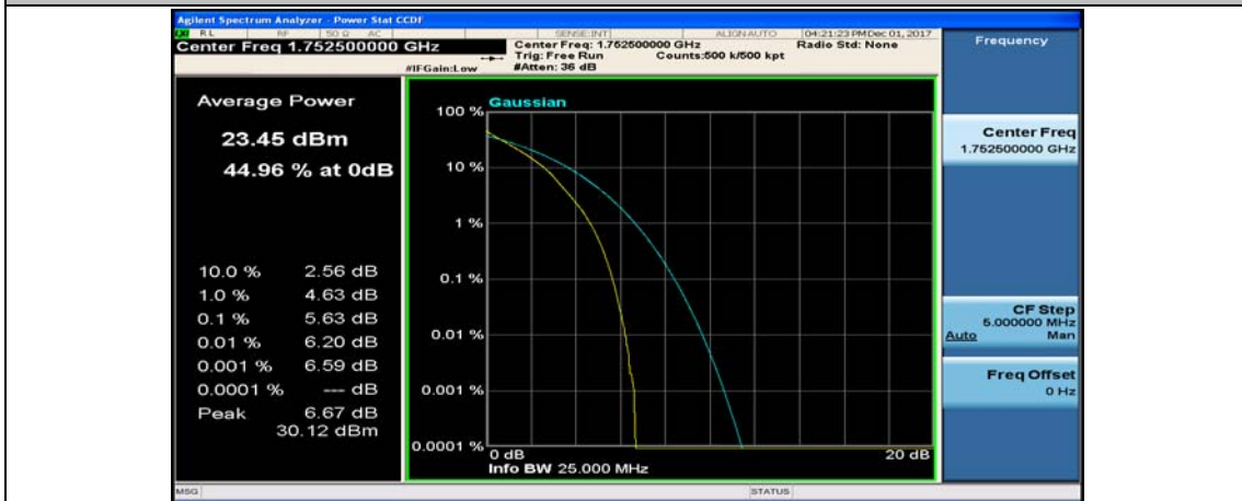
(Channel Bandwidth: 5 MHz)_HCH_QPSK_25RB#0
