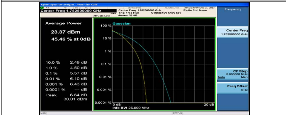
(Channel Bandwidth: 5 MHz)_HCH_QPSK_25RB#0
