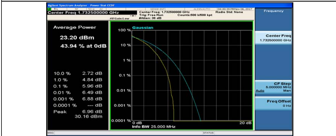
(Channel Bandwidth: 1.4 MHz)_MCH_QPSK_6RB#0
