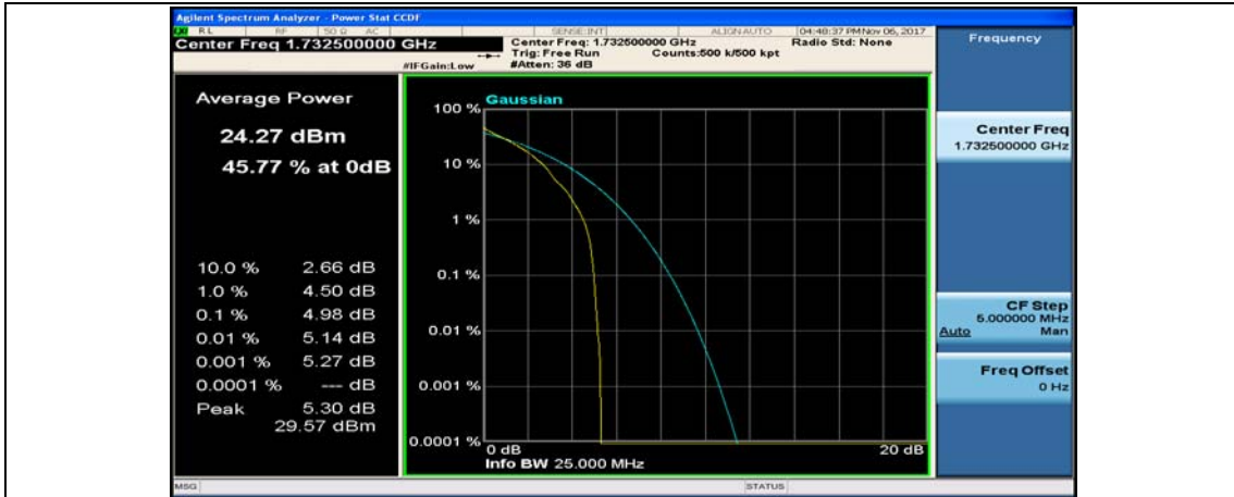
(Channel Bandwidth: 1.4 MHz)_MCH_QPSK_3RB#0
