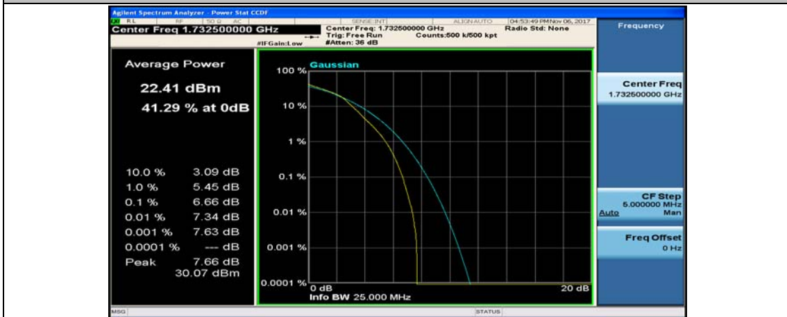
(Channel Bandwidth: 3 MHz)_MCH_16QAM_8RB#7
