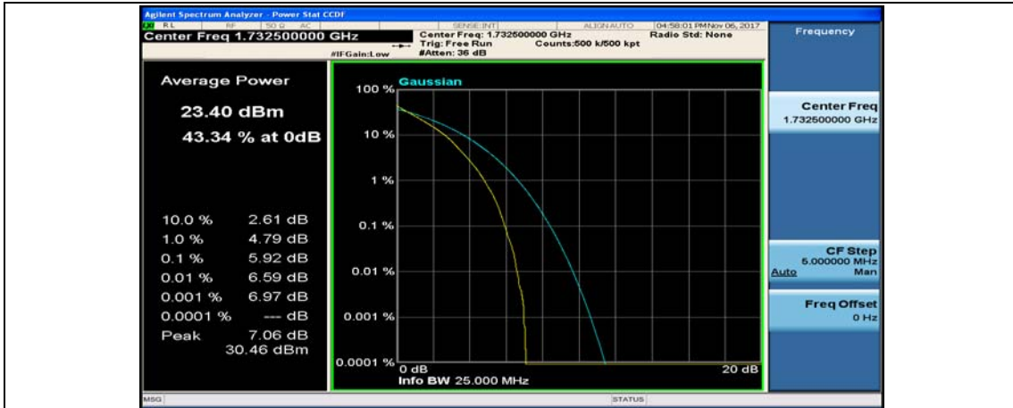
(Channel Bandwidth: 5 MHz)_MCH_QPSK_25RB#0
