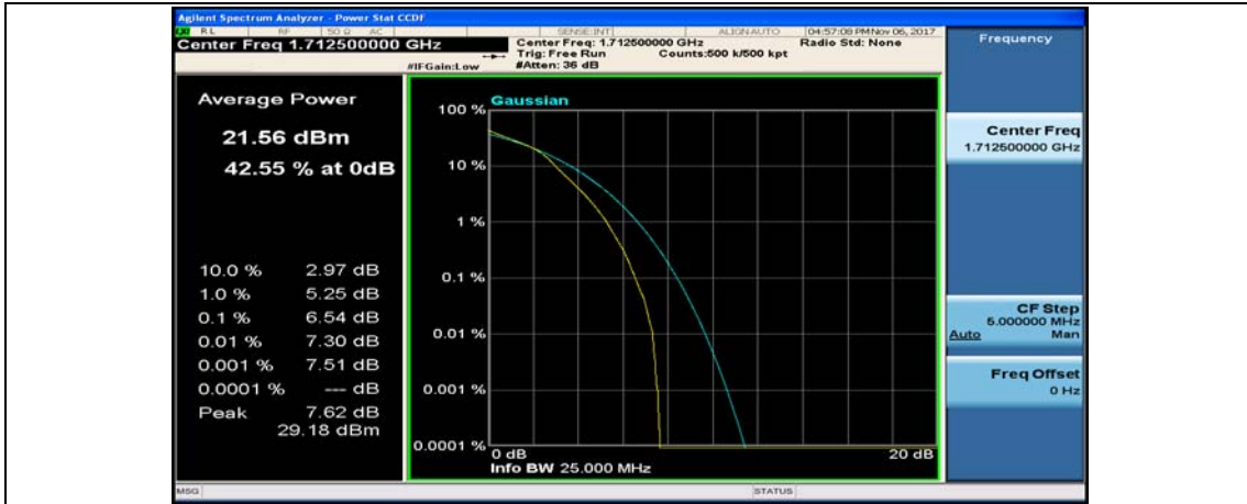
(Channel Bandwidth: 5 MHz)_MCH_16QAM_1RB#0
