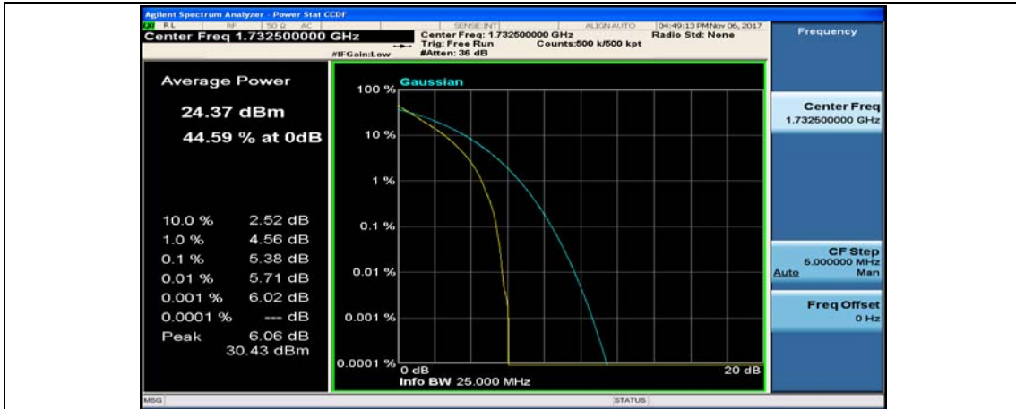
(Channel Bandwidth: 1.4 MHz)_MCH_QPSK_6RB#0
