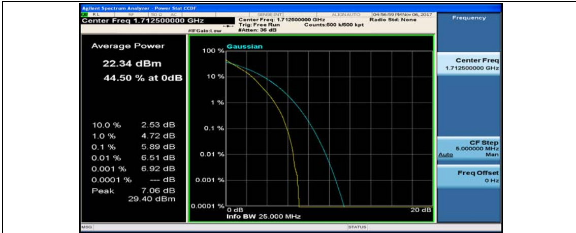
(Channel Bandwidth: 5 MHz)_MCH_QPSK_1RB#0
