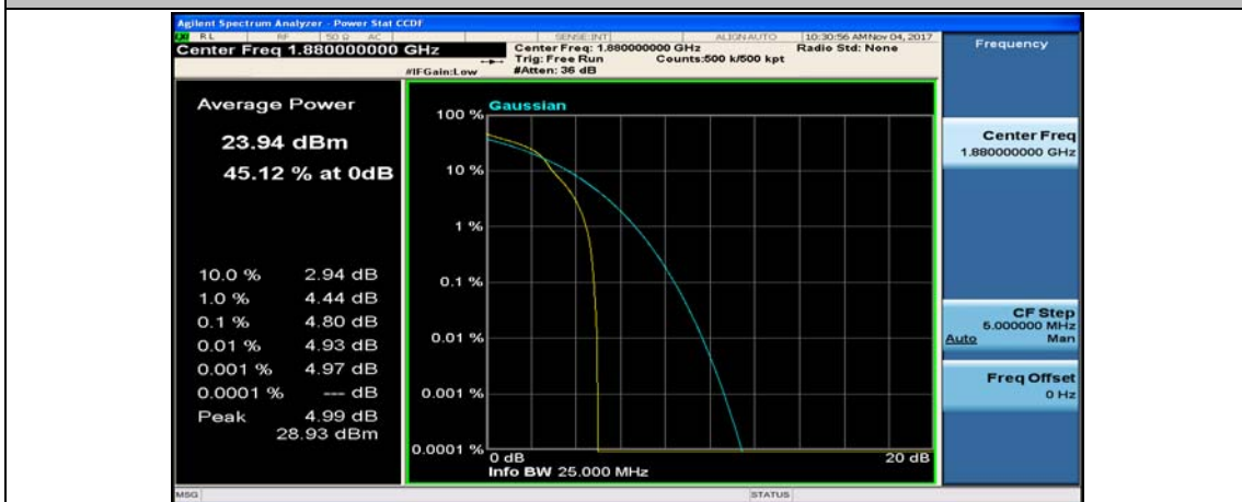
Channel Bandwidth: 10 MHz_MCH_16QAM_1RB#49
