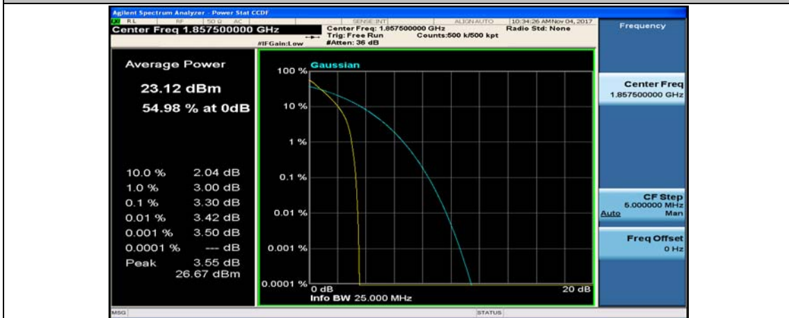
(Channel Bandwidth:15 MHz)_LCH_QPSK_75RB#0
