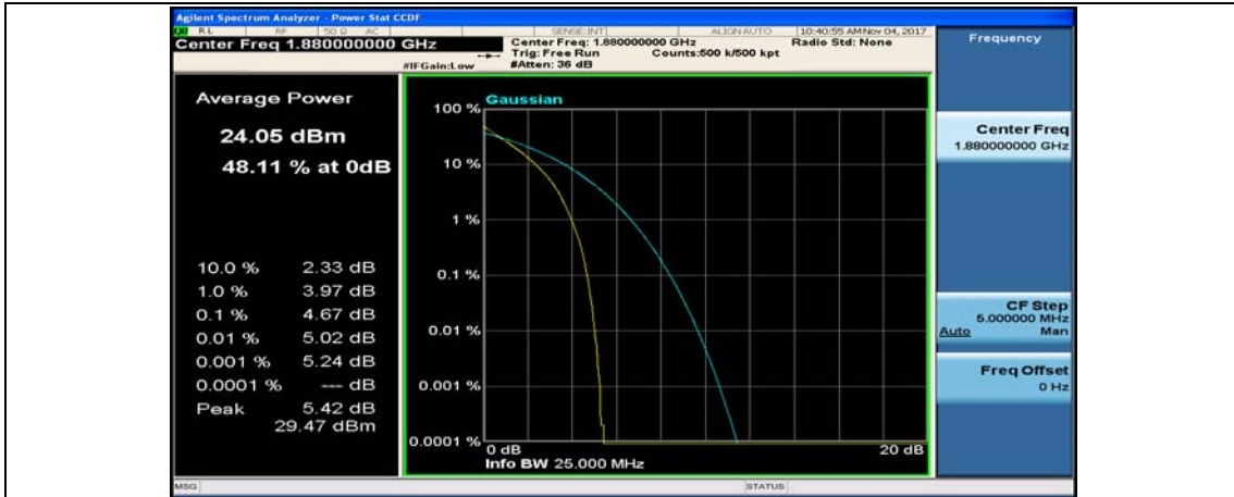
(Channel Bandwidth:20 MHz)_MCH_QPSK_100RB#0
