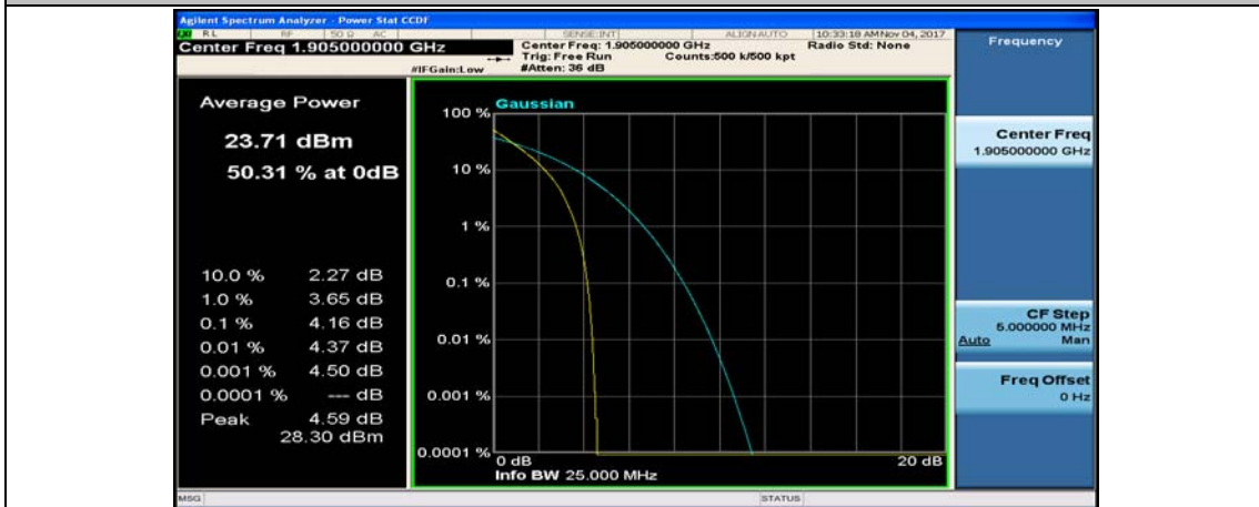
Channel Bandwidth: 10 MHz_LCH_16QAM_1RB#0
