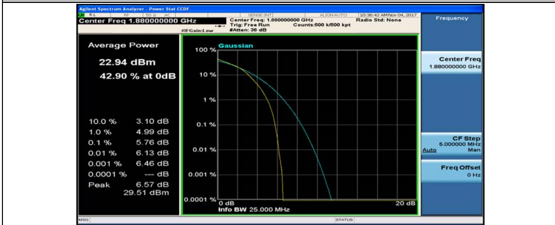
(Channel Bandwidth:15 MHz)_MCH_16QAM_75RB#0
