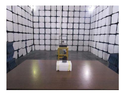
Spurious Radiation Test Setup (30MHz to 1G)
