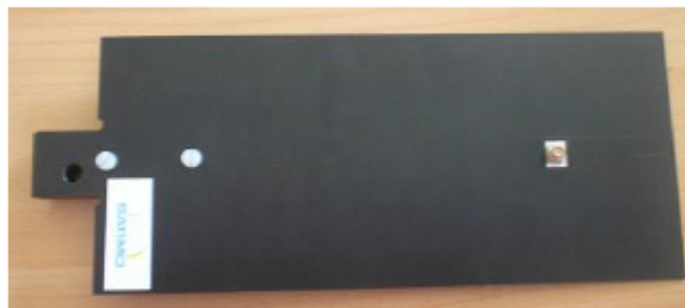
Figure 1 – MVG COMOHAC Validation Dipole
