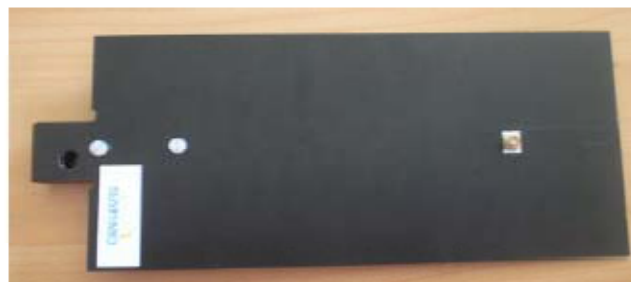
Figure 1 – MVG COMOHAC Validation Dipole
