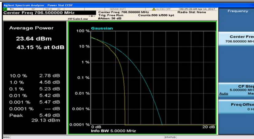
(Channel Bandwidth: 5 MHz)_LCH_QPSK_1RB#24
