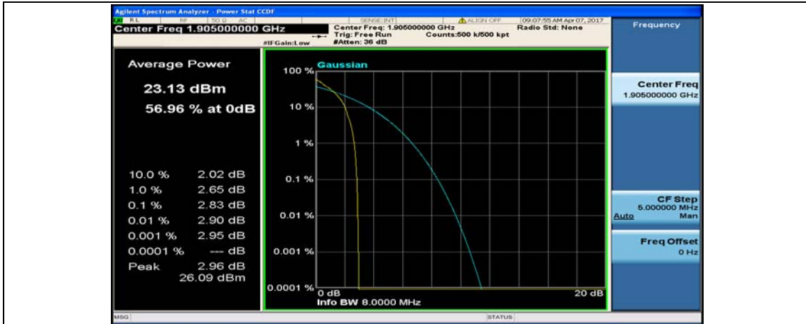
Channel Bandwidth: 10 MHz_HCH_QPSK_1RB#49
