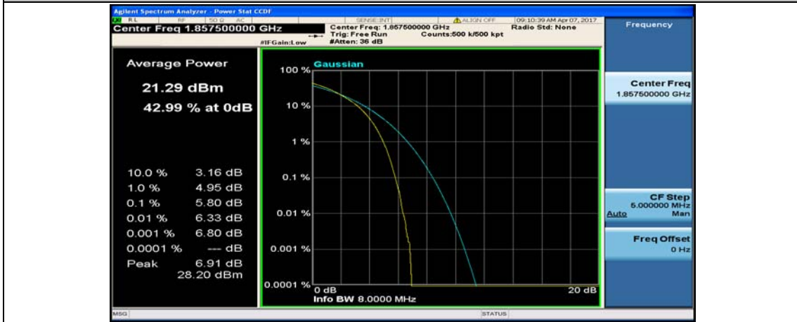
(Channel Bandwidth:15 MHz)_LCH_16QAM_75RB#0
