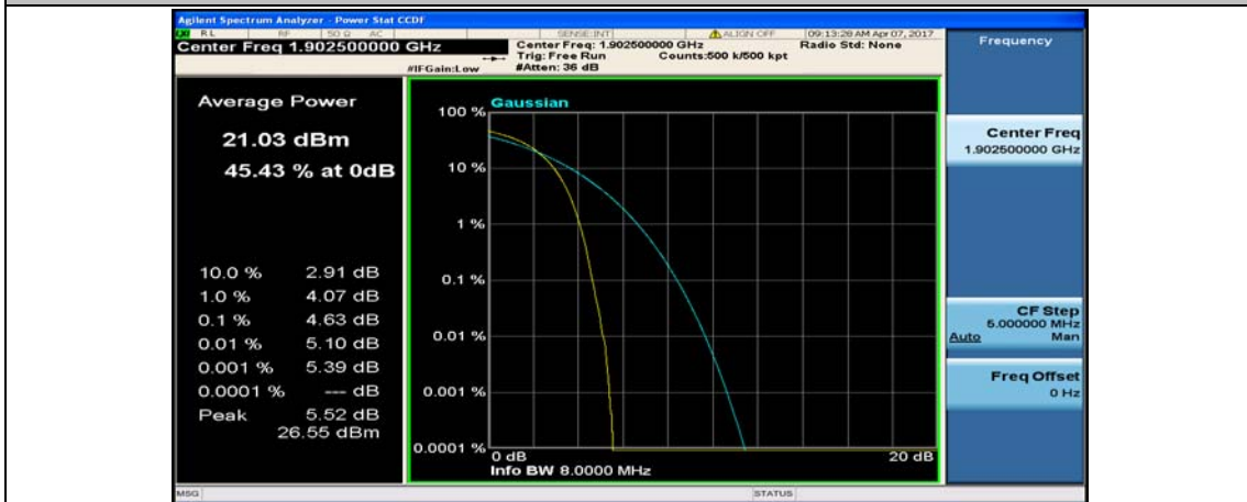
(Channel Bandwidth:15 MHz)_HCH_QPSK_37RB#18
