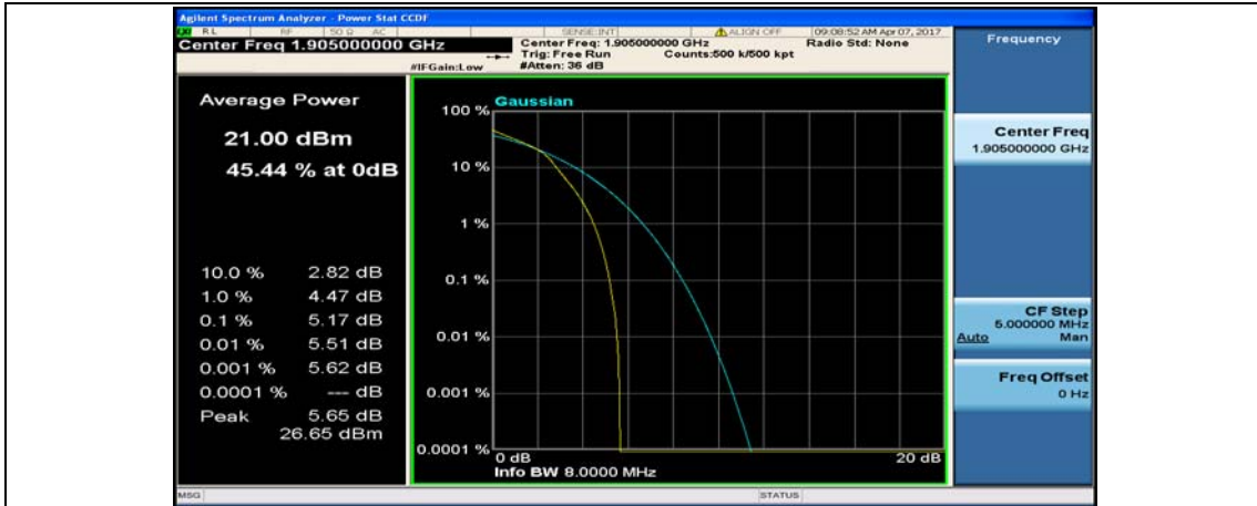
Channel Bandwidth: 10 MHz_HCH_16QAM_25RB#25
