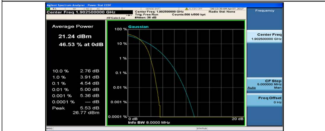
(Channel Bandwidth:15 MHz)_HCH_QPSK_75RB#0
