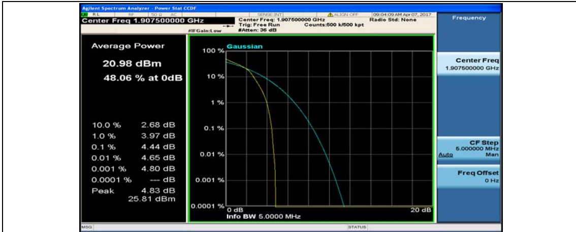
(Channel Bandwidth: 5 MHz)_HCH_16QAM_12RB#13
