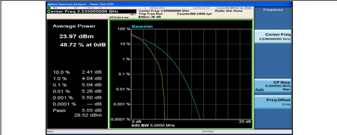
(Channel Bandwidth: 5 MHz)_MCH_QPSK_12RB#0
