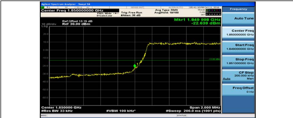
(Channel Bandwidth: 3 MHz)_LCH_16QAM_8RB#4
