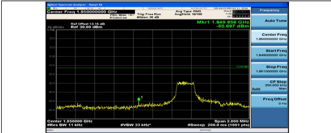
(Channel Bandwidth: 5 MHz)_LCH_16QAM_12RB#0
