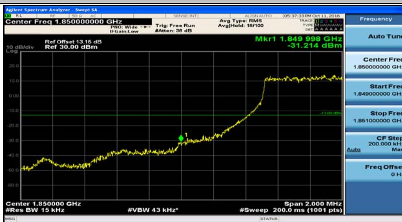
(Channel Bandwidth: 1.4 MHz)_LCH_QPSK_3RB#3
