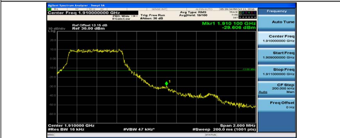
(Channel Bandwidth: 1.4 MHz)_HCH_16QAM_3RB#3
