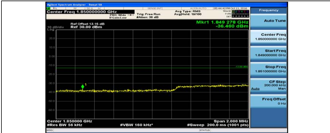
(Channel Bandwidth: 5 MHz)_LCH_16QAM_25RB#0
