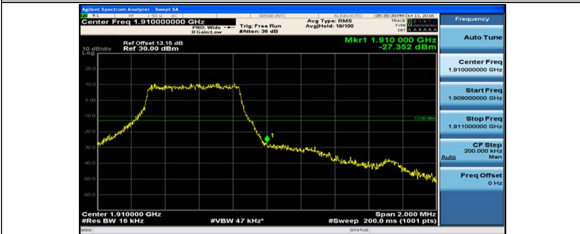
(Channel Bandwidth: 1.4 MHz)_HCH_16QAM_6RB#0
