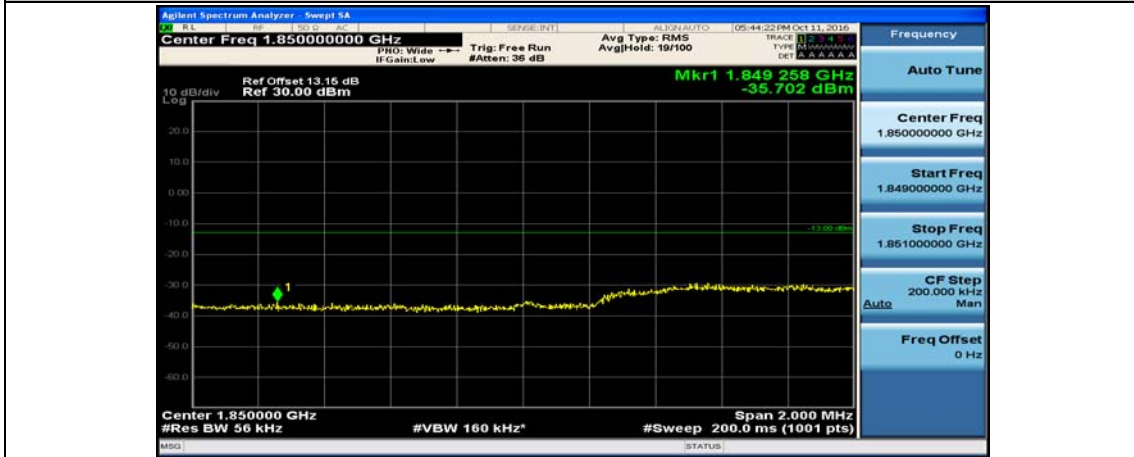
(Channel Bandwidth: 5 MHz)_LCH_QPSK_25RB#0
