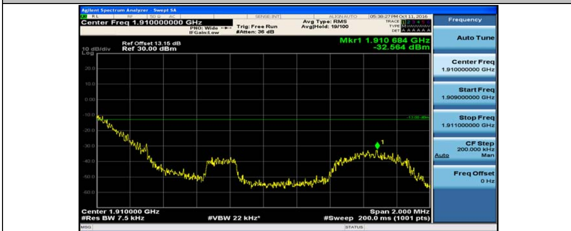
(Channel Bandwidth: 1.4 MHz)_HCH_QPSK_1RB#3
