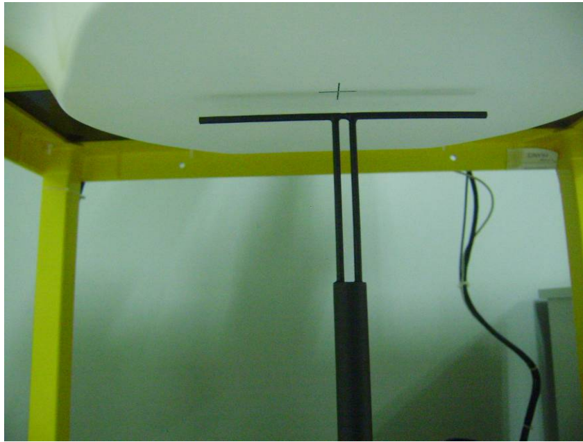
Setup Photo of Dipole Antenna
