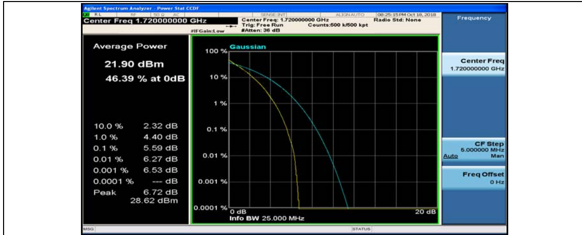
(Channel Bandwidth:20 MHz)_MCH_QPSK_1RB#0
