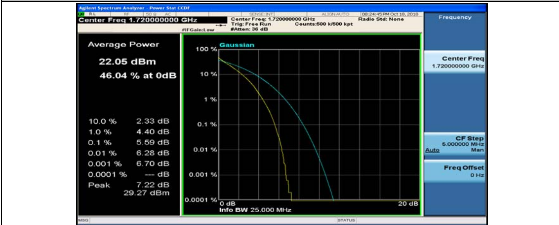
(Channel Bandwidth:20 MHz)_LCH_QPSK_100RB#0
