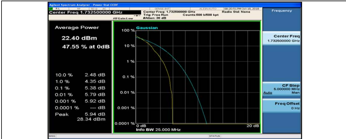
(Channel Bandwidth:15 MHz)_MCH_QPSK_37RB#0
