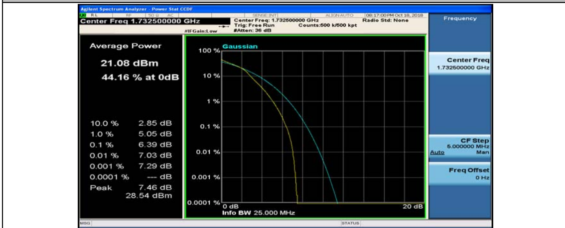
Channel Bandwidth: 10 MHz_MCH_16QAM_25RB#25
