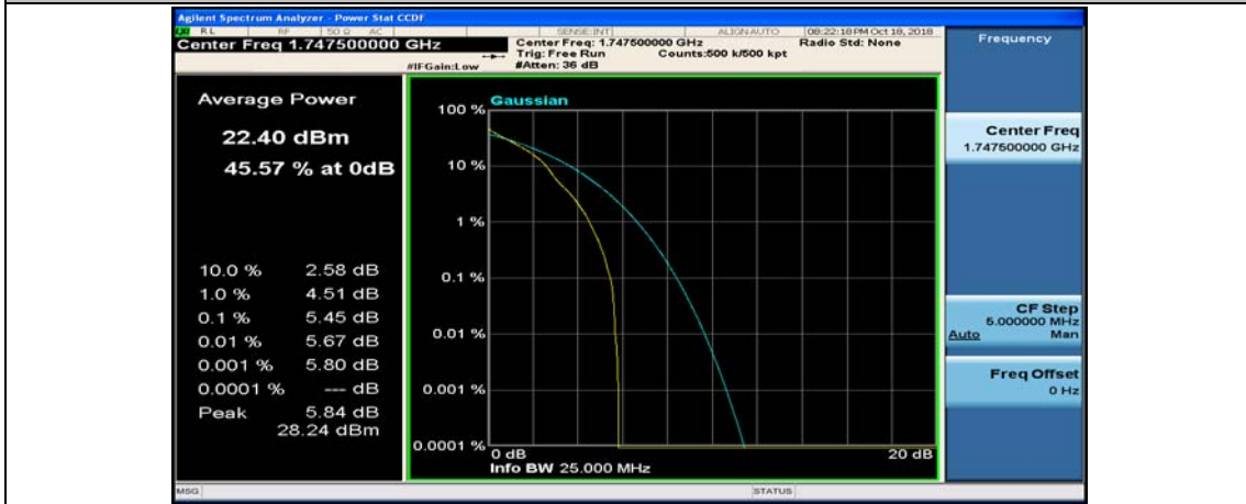
(Channel Bandwidth:15 MHz)_HCH_QPSK_1RB#37
