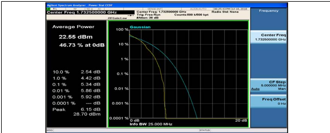
(Channel Bandwidth:20 MHz)_MCH_QPSK_50RB#0
