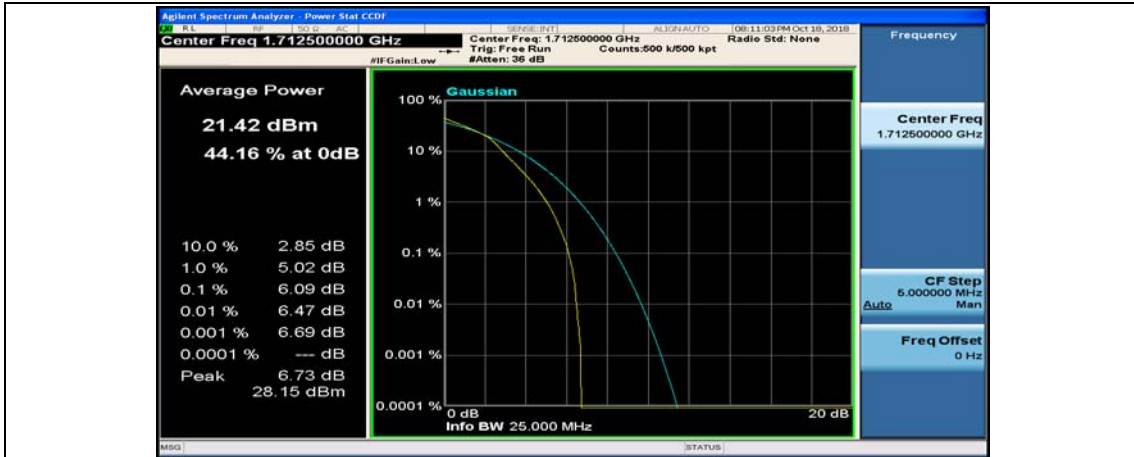
(Channel Bandwidth: 5 MHz)_LCH_16QAM_12RB#6
