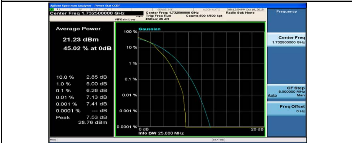
(Channel Bandwidth: 5 MHz)_MCH_16QAM_25RB#0
