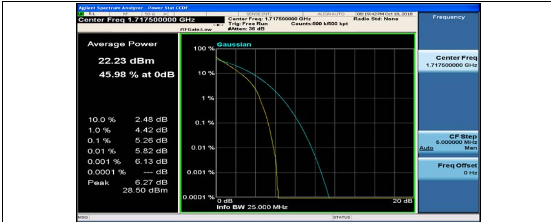
(Channel Bandwidth:15 MHz)_LCH_QPSK_37RB#18
