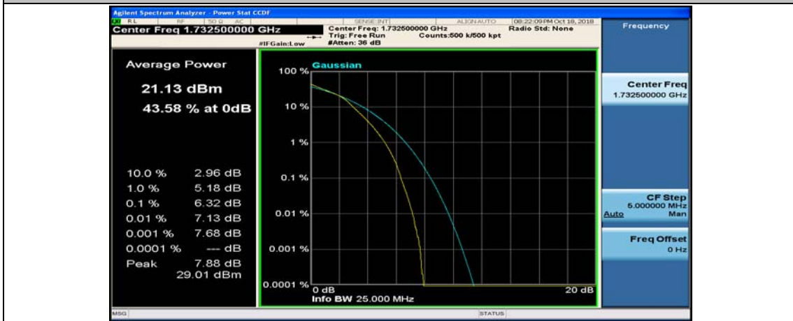
(Channel Bandwidth:15 MHz)_MCH_16QAM_75RB#0
