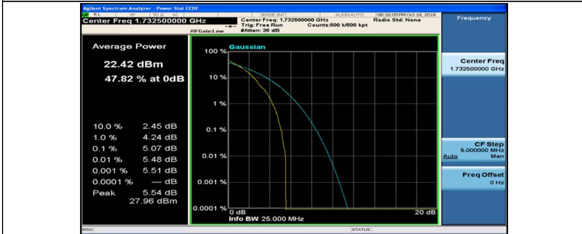
Channel Bandwidth: 10 MHz_MCH_QPSK_1RB#49
