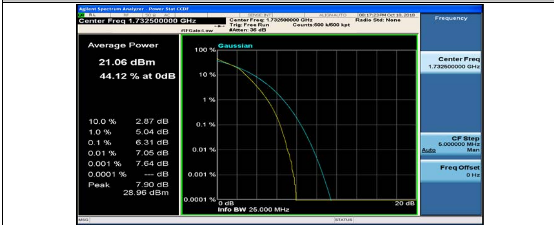
Channel Bandwidth: 10 MHz_MCH_16QAM_50RB#0
