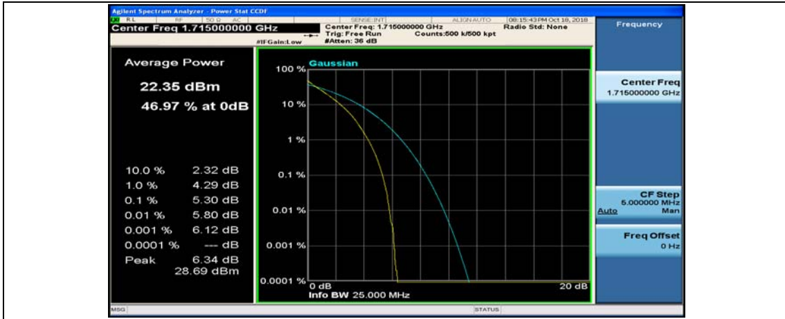
Channel Bandwidth: 10 MHz_MCH_QPSK_1RB#0
