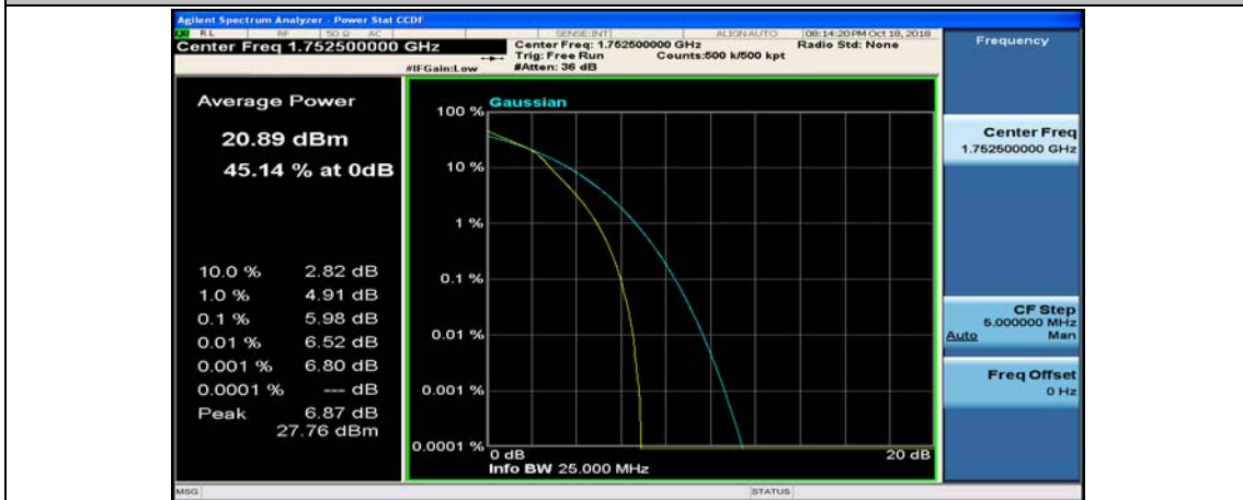
(Channel Bandwidth: 5 MHz)_HCH_16QAM_25RB#0
