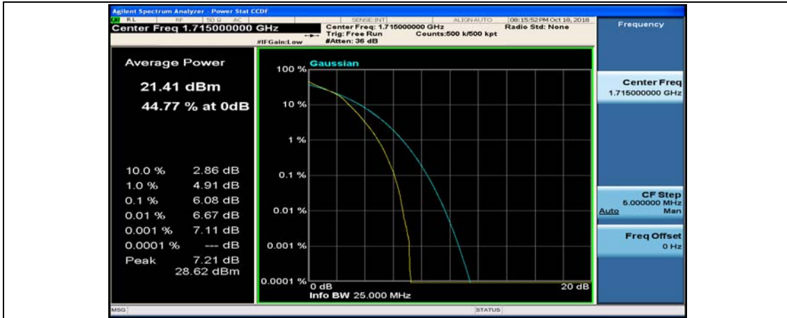
Channel Bandwidth: 10 MHz_MCH_16QAM_1RB#0
