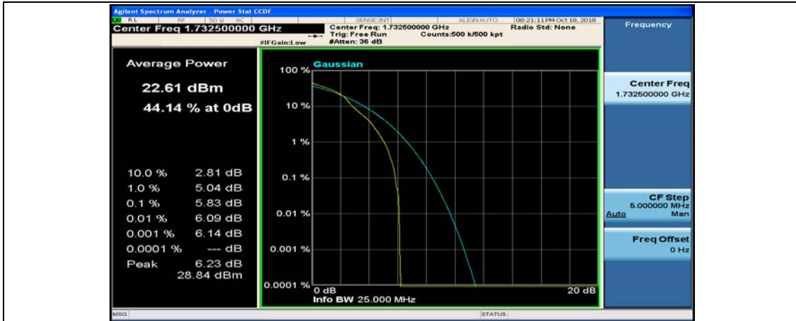
(Channel Bandwidth:15 MHz)_MCH_16QAM_37RB#0
