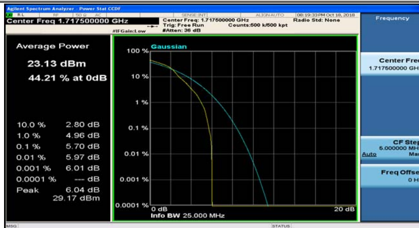
(Channel Bandwidth:15 MHz)_LCH_16QAM_37RB#0
