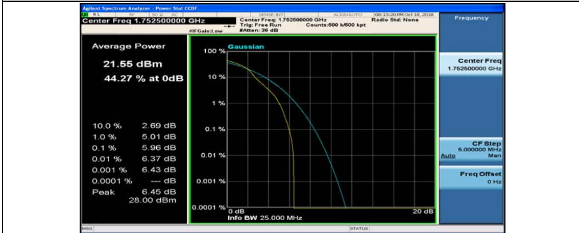
(Channel Bandwidth: 5 MHz)_HCH_16QAM_1RB#12
