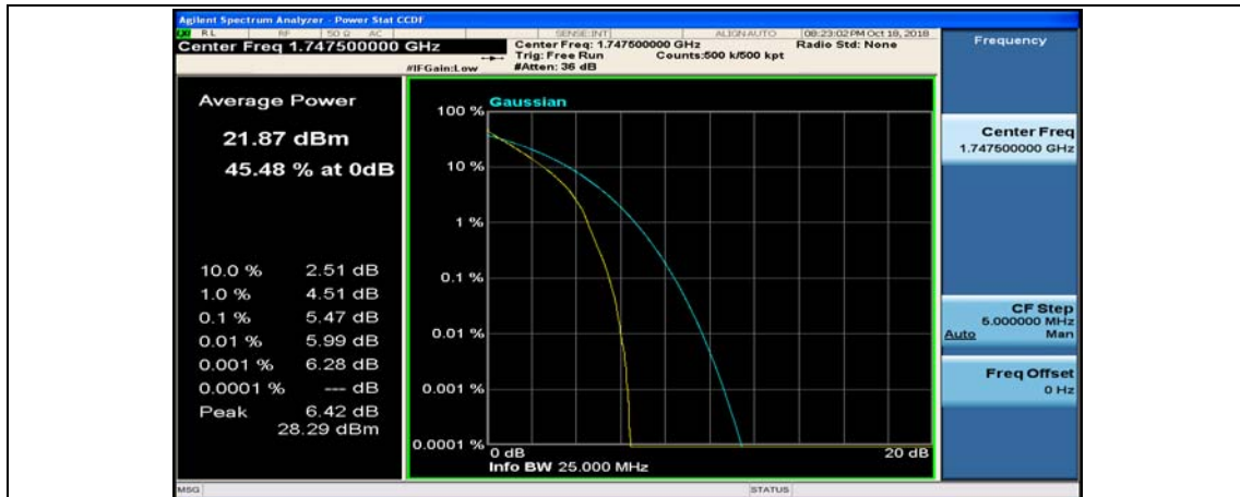
(Channel Bandwidth:15 MHz)_HCH_QPSK_37RB#38
