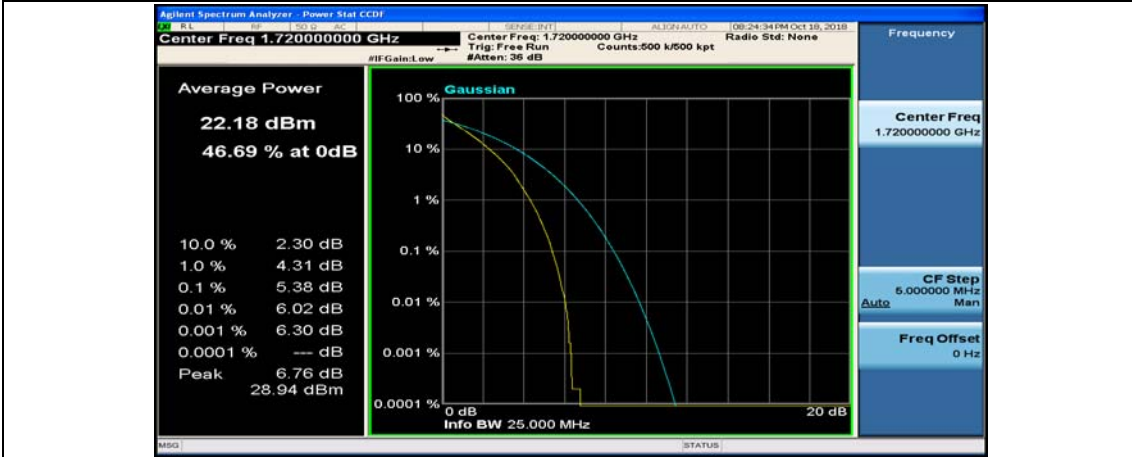
(Channel Bandwidth:20 MHz)_LCH_QPSK_50RB#25
