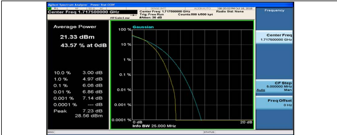
(Channel Bandwidth:15 MHz)_LCH_16QAM_37RB#18
