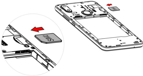
2. The SD card should be installed in the upper part of the SIM card 2.
