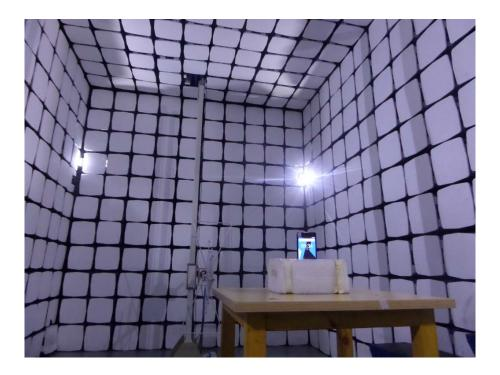
Radiation Emission Test Setup (Above 1GHz)
