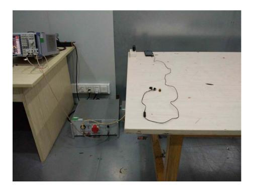
Radiation Emission Test Setup (Below 30MHz)
