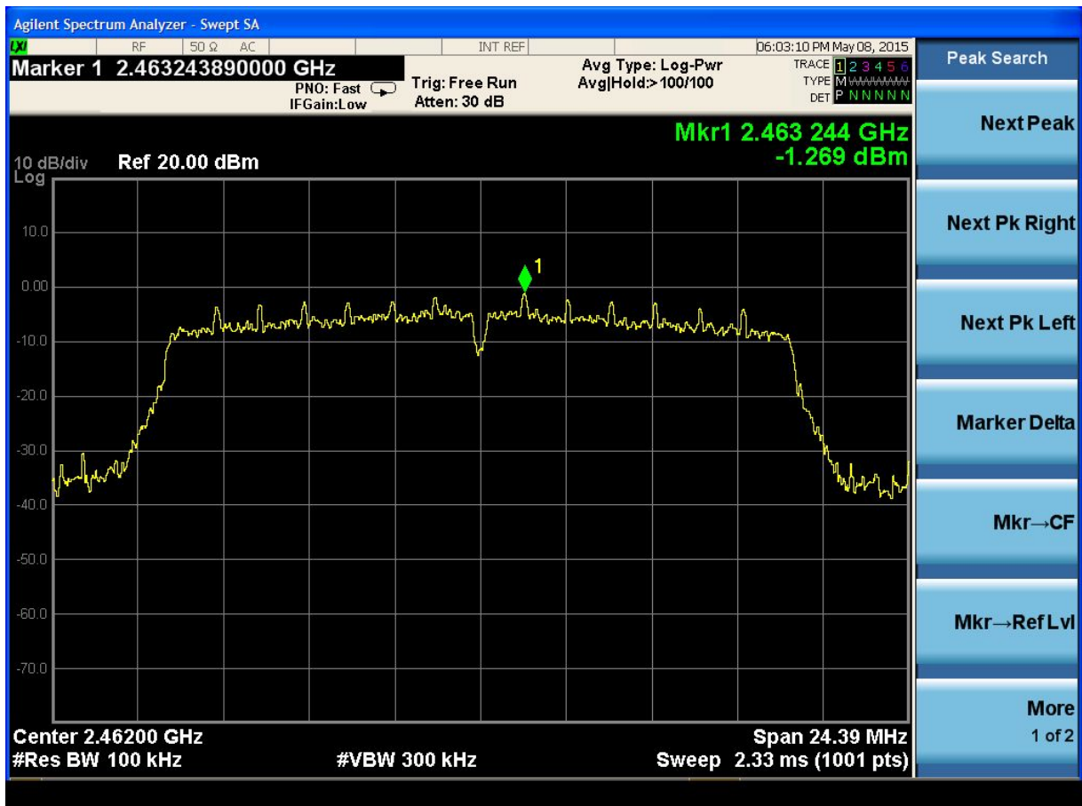
(Plot 4.6.3 C1: Channel 11: 2462MHz @ 802.11n HT20)
