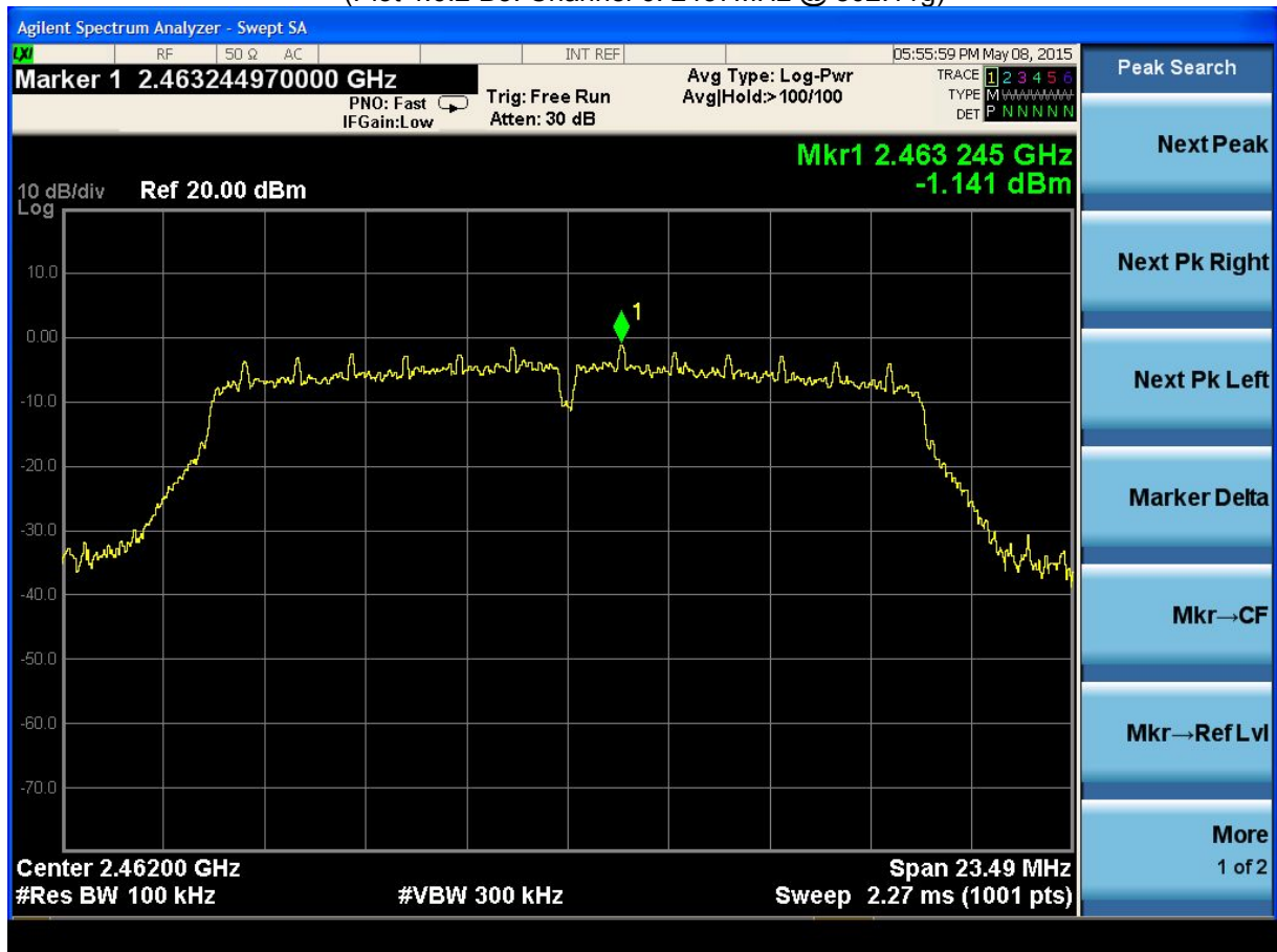
(Plot 4.6.2 C1: Channel 11: 2462MHz @ 802.11g)
