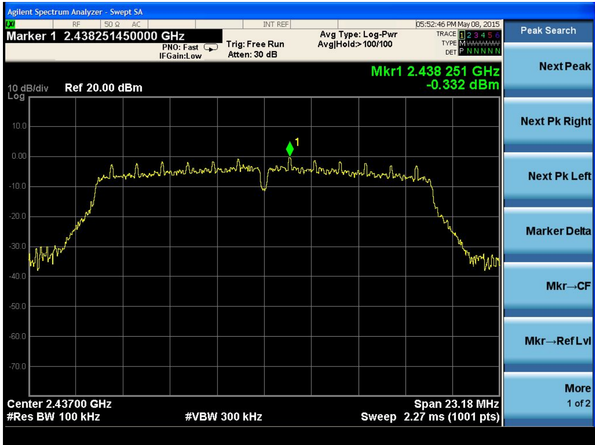
(Plot 4.6.2 B1: Channel 6: 2437MHz @ 802.11g)
