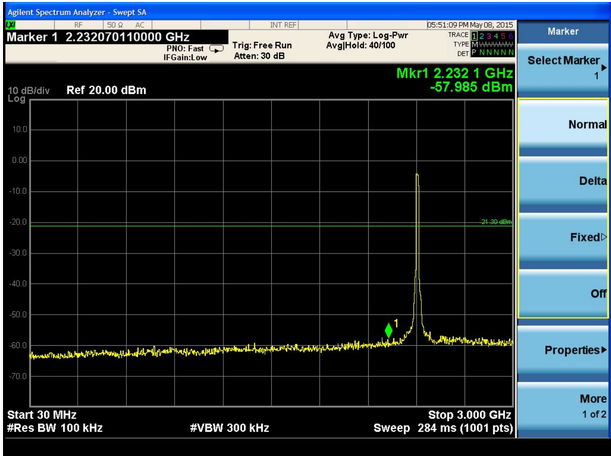
(Plot 4.6.2 A2: Channel 1: 2412MHz @ 802.11g)
