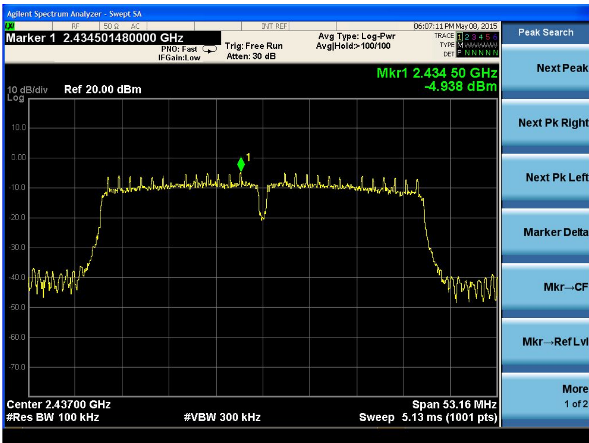
(Plot 4.4.4 B: Channel 6: 2437MHz @ 802.11n HT40)
