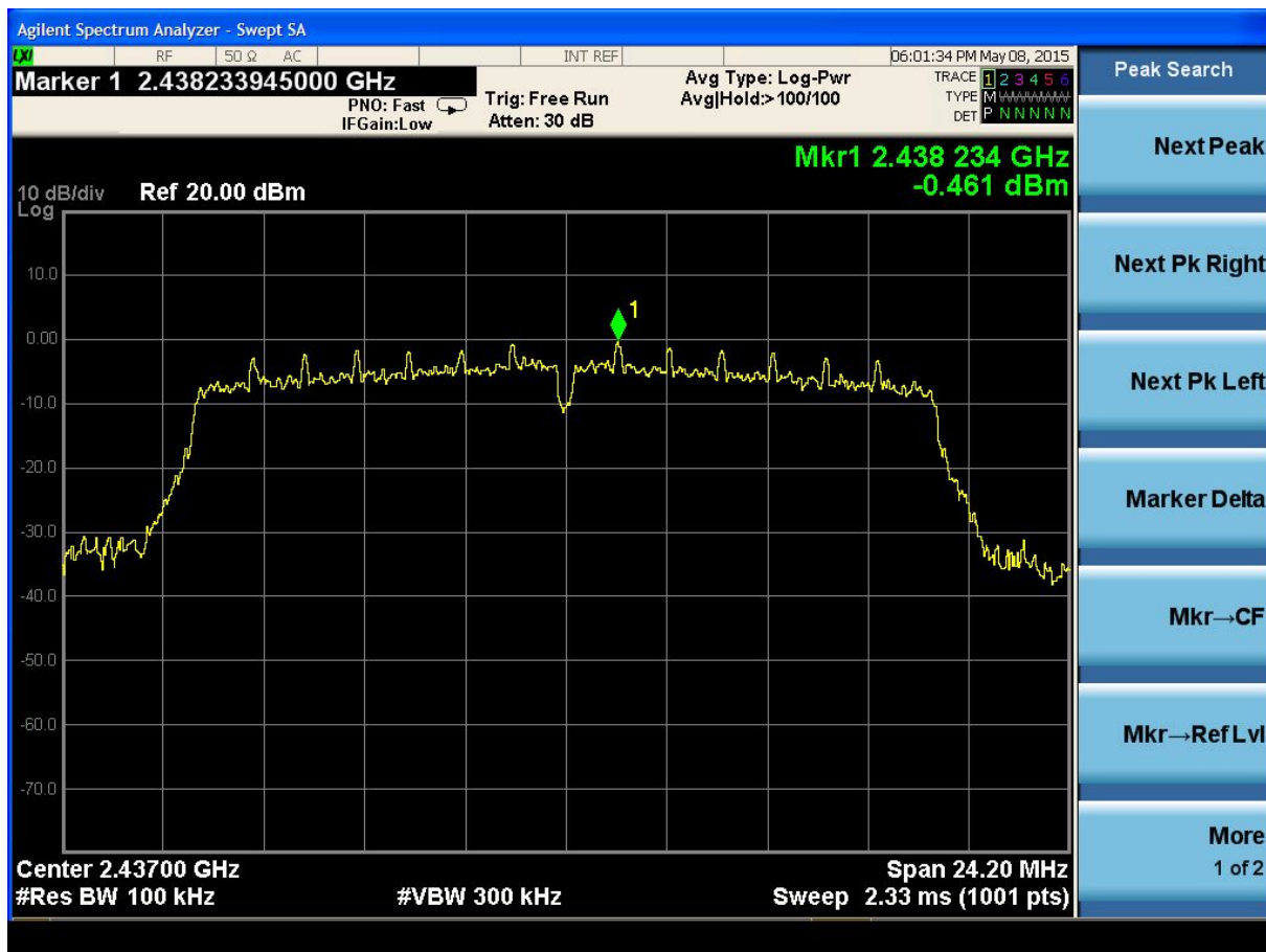
(Plot 4.4.3 B: Channel 6: 2437MHz @ 802.11n HT20)
