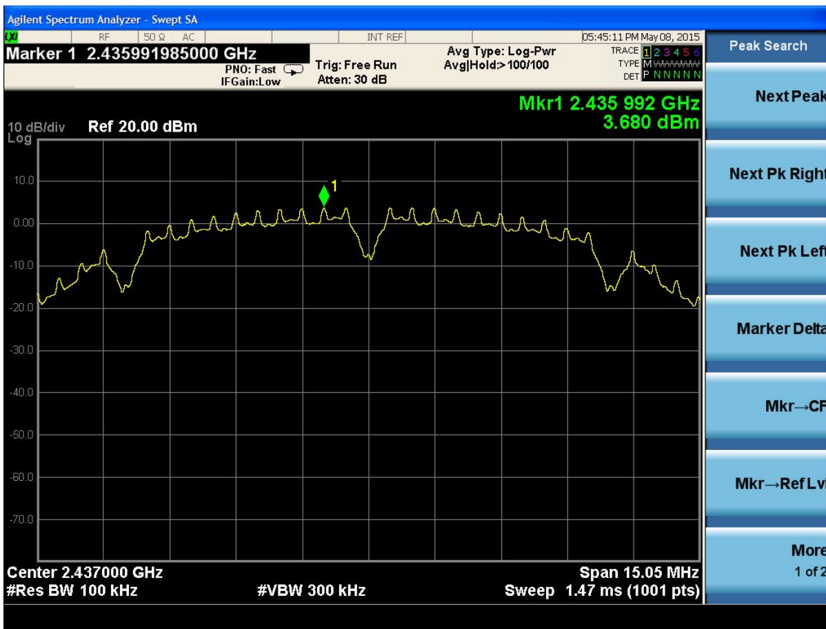
(Plot 4.4.1 B: Channel 6: 2437MHz @ 802.11b)
