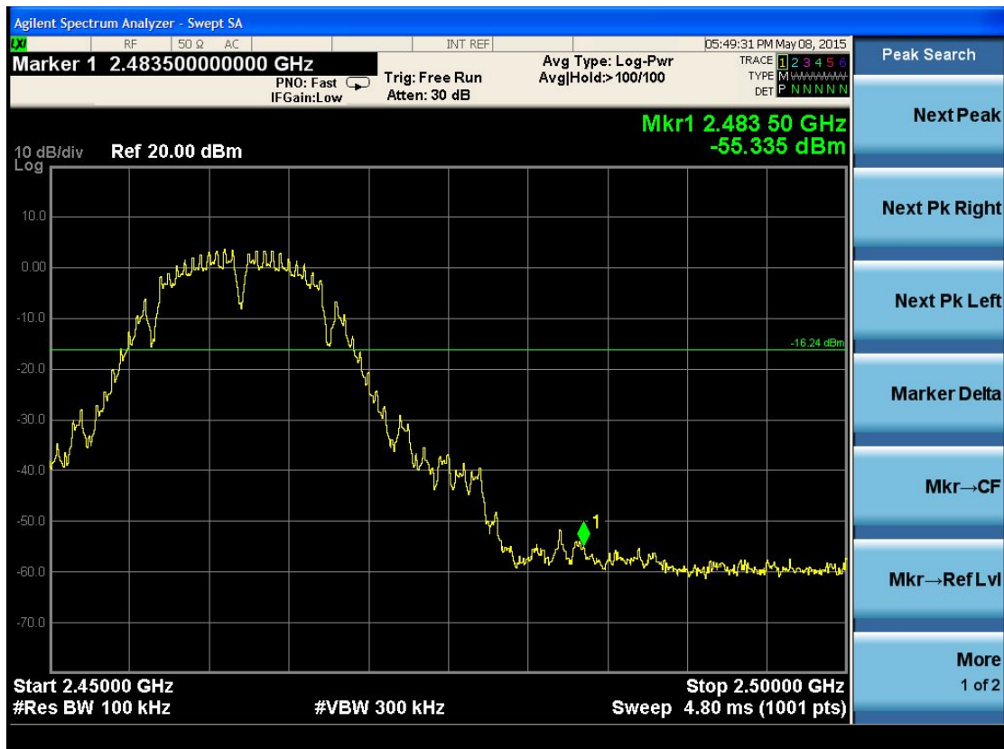
(Plot 4.5.2.1 B: Channel 11: 2462MHz @ 802.11 b )
