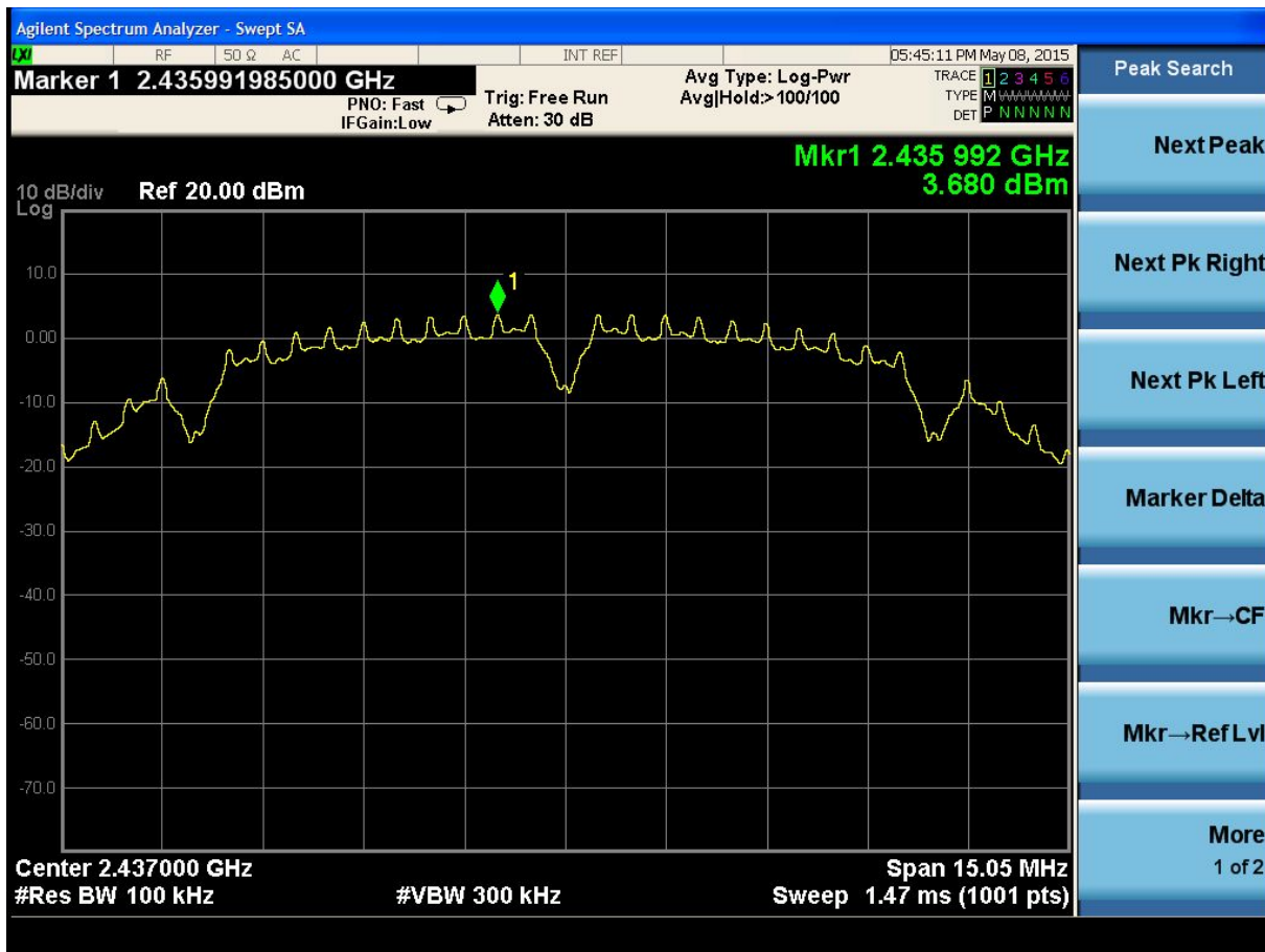
(Plot 4.6.1 B1: Channel 6: 2437MHz @ 802.11b)
