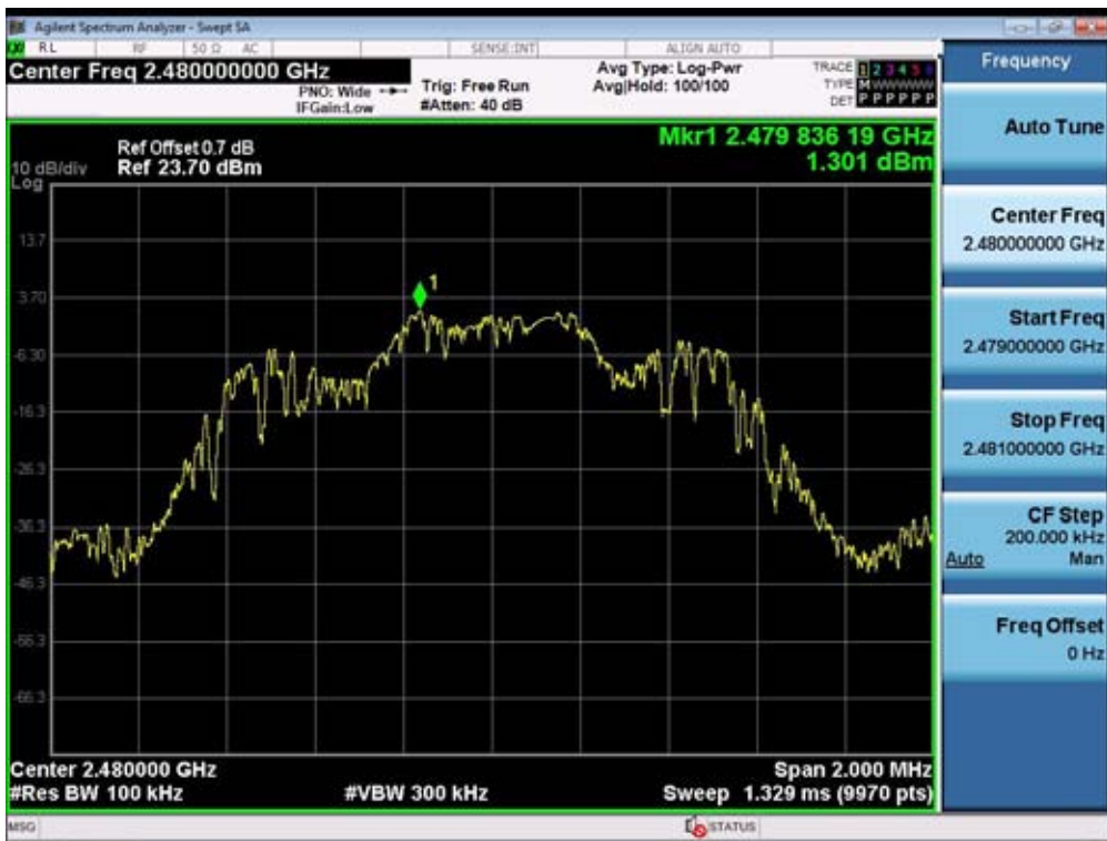
(Plot 4.9.2 C1: Channel 78: 2480MHz @ \pi/4 DQPSK)
