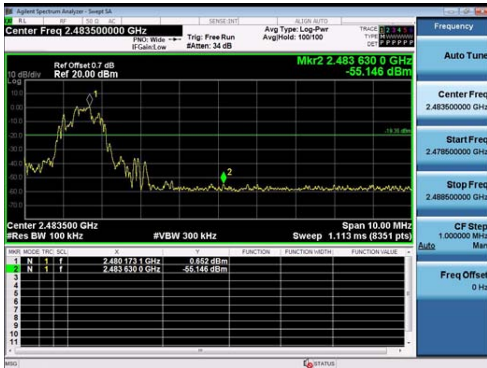
(Plot 4.5.2.2 B: Hopping Mode @ 8DPSK)
