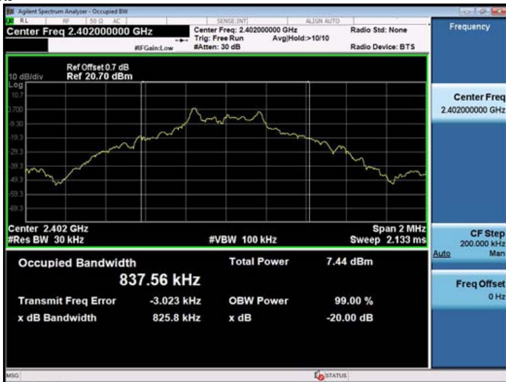
(Plot 4.4.1 A: Channel 00: 2402MHz @ GFSK)
