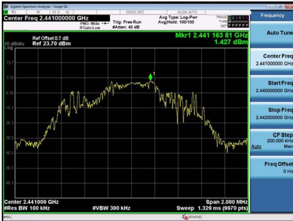
(Plot 4.9.3 B1: Channel 39: 2441MHz @ 8DPSK)
