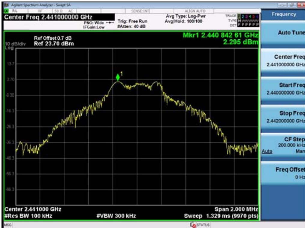
(Plot 4.9.1 B1: Channel 39: 2441MHz @ GFSK)
