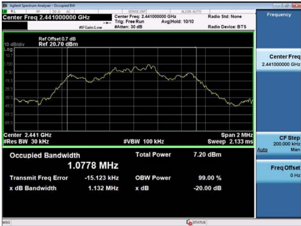
(Plot 4.4.2 B: Channel 39: 2441MHz @ 8DPSK)
