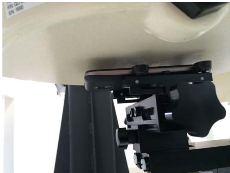
10mm Body-worn Front Side Setup Photo
