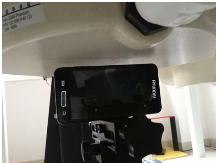
10mm Body-worn Right Side Setup Photo
