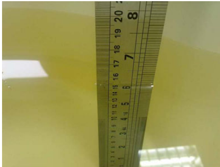
Photograph of the depth in the Head Phantom (850MHz)
