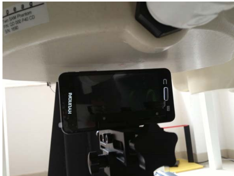
10mm Body-worn Left Side Setup Photo
