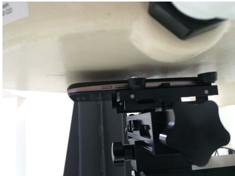
10mm Body-worn Rear Side Setup Photo
