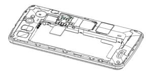
3. Put the SD card into card slot.
