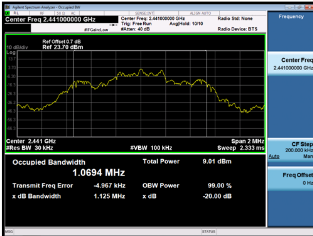
(Plot 4.4.3 B: Channel 39: 2441MHz @ \pi/4 DQPSK)
