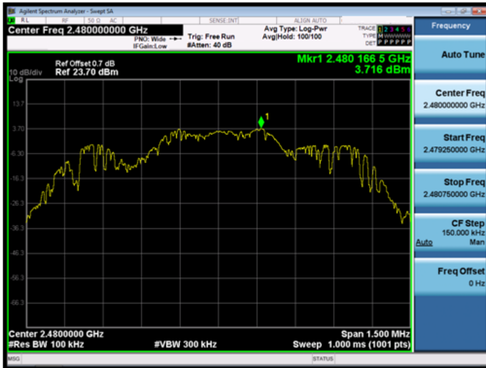
(Plot 4.9.3 C1: Channel 78: 2480MHz @ 8DPSK)
