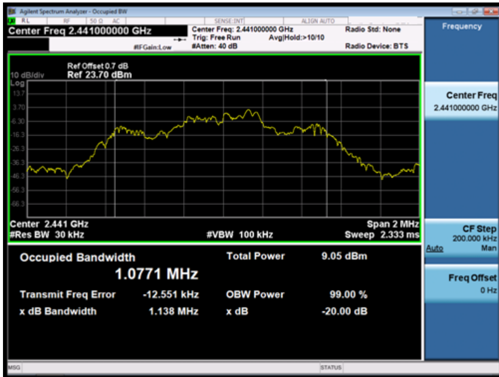
(Plot 4.4.2 B: Channel 39: 2441MHz @ 8DPSK)
