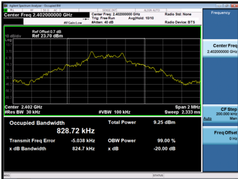
(Plot 4.4.1 A: Channel 00: 2402MHz @ GFSK)
