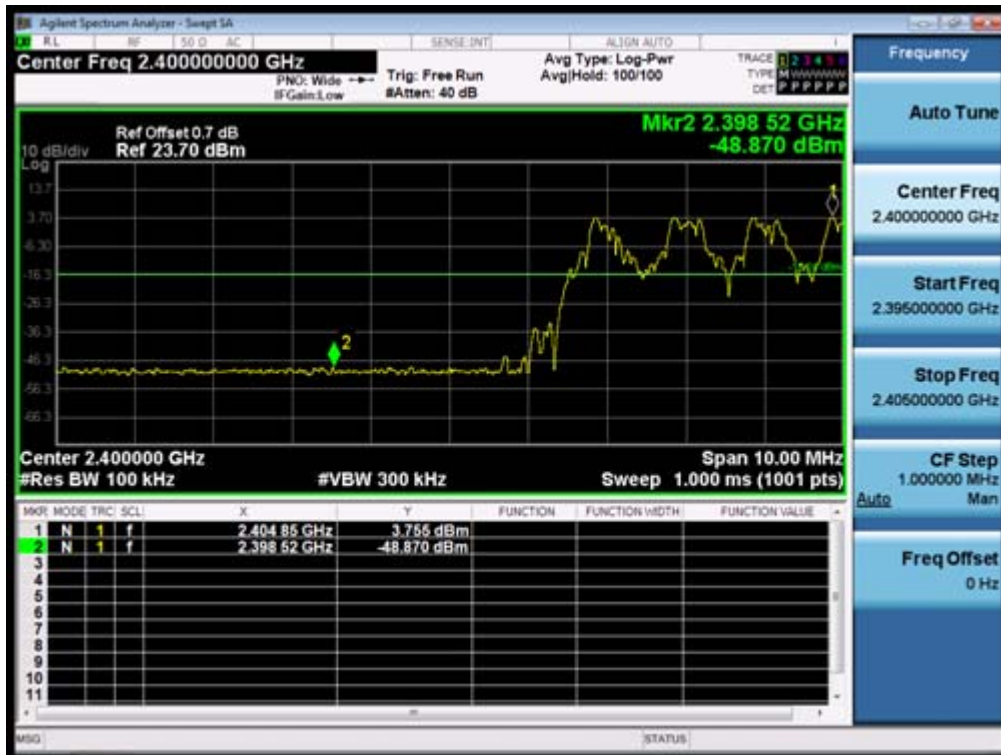
(Plot 4.5.2.1 B: Hopping Mode @ GFSK)
