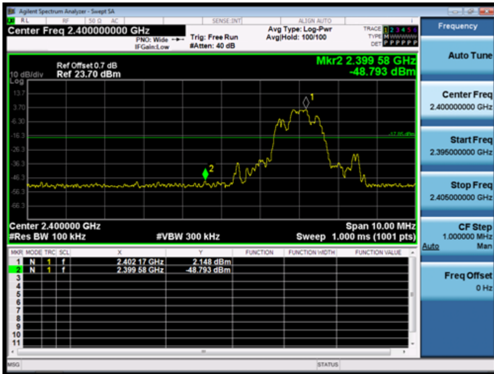
(Plot 4.5.2.2 A: Channel 00: 2402MHz @ 8DPSK)
