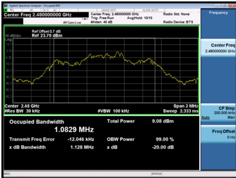
(Plot 4.4.2 C: Channel 78: 2480MHz @ 8DPSK)
