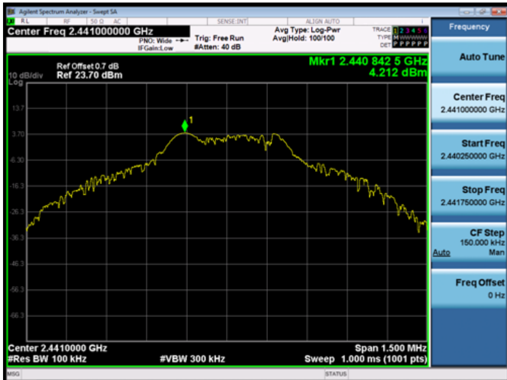
(Plot 4.9.1 B1: Channel 39: 2441MHz @ GFSK)
