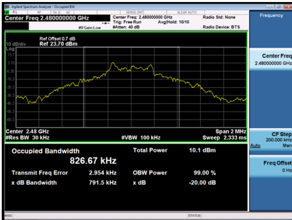
(Plot 4.4.1 C: Channel 78: 2480MHz @ GFSK)
