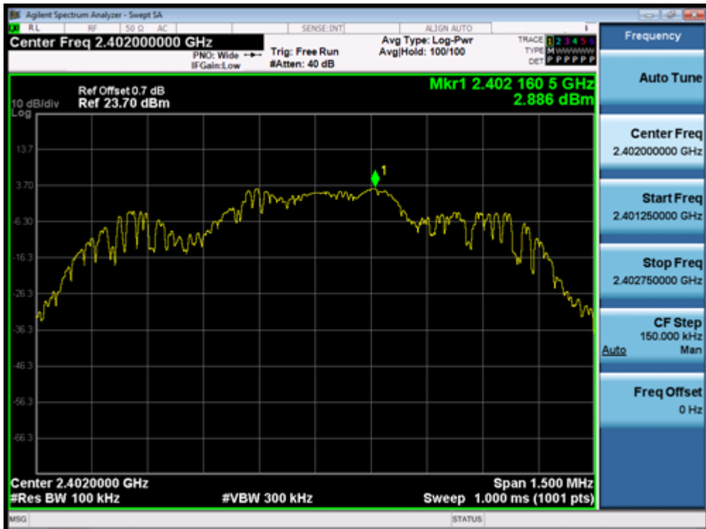
(Plot 4.9.3 A1: Channel 00: 2402MHz @ 8DPSK)
