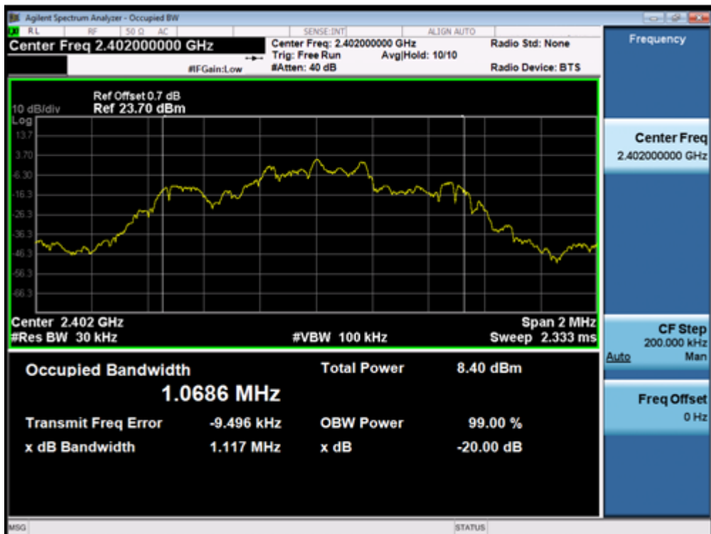
(Plot 4.4.3 A: Channel 00: 2402MHz @ \pi/4 DQPSK)
