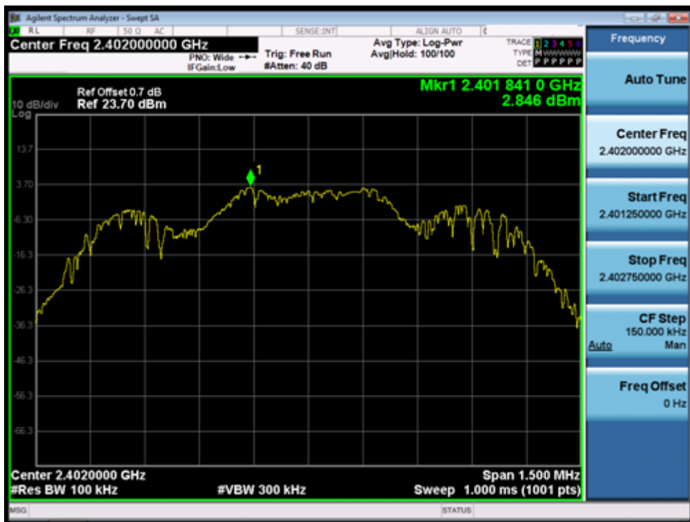
(Plot 4.9.2 A1: Channel 00: 2402MHz @ \pi/4 DQPSK)
