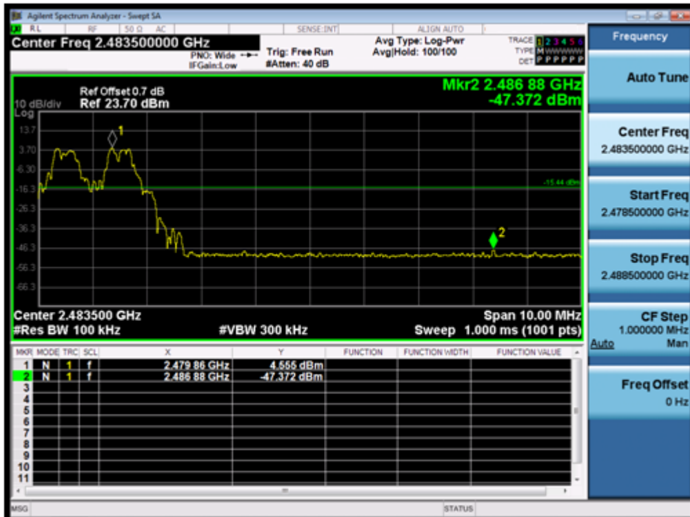
(Plot 4.5.2.1 D: Hopping Mode @ GFSK)
