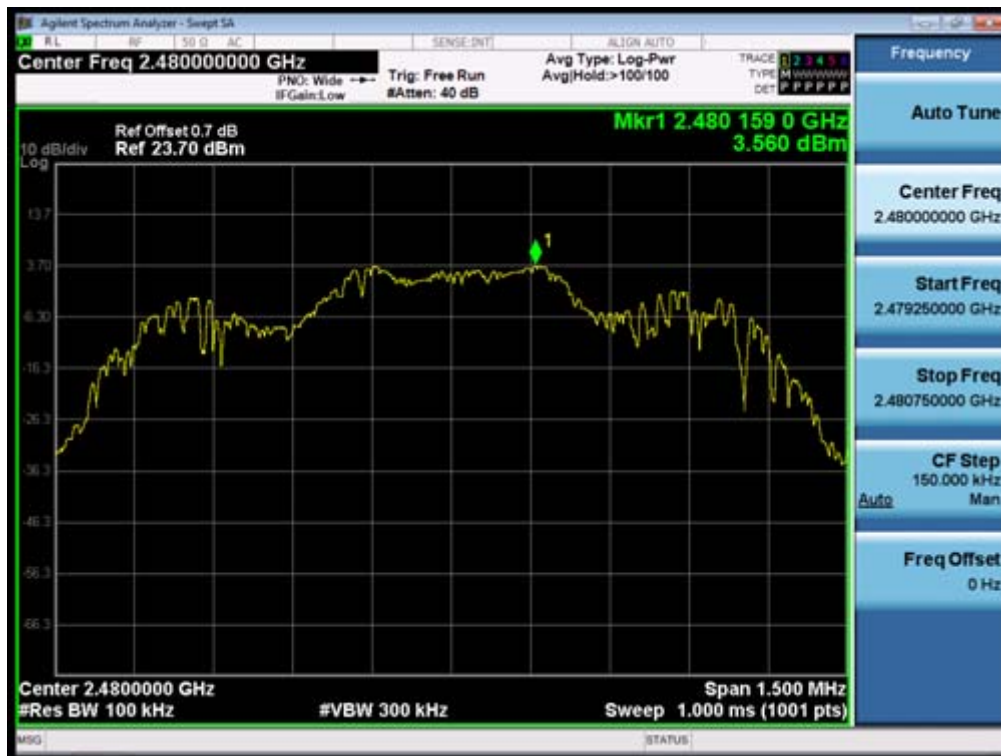
(Plot 4.9.2 C1: Channel 78: 2480MHz @ \pi/4 DQPSK)
