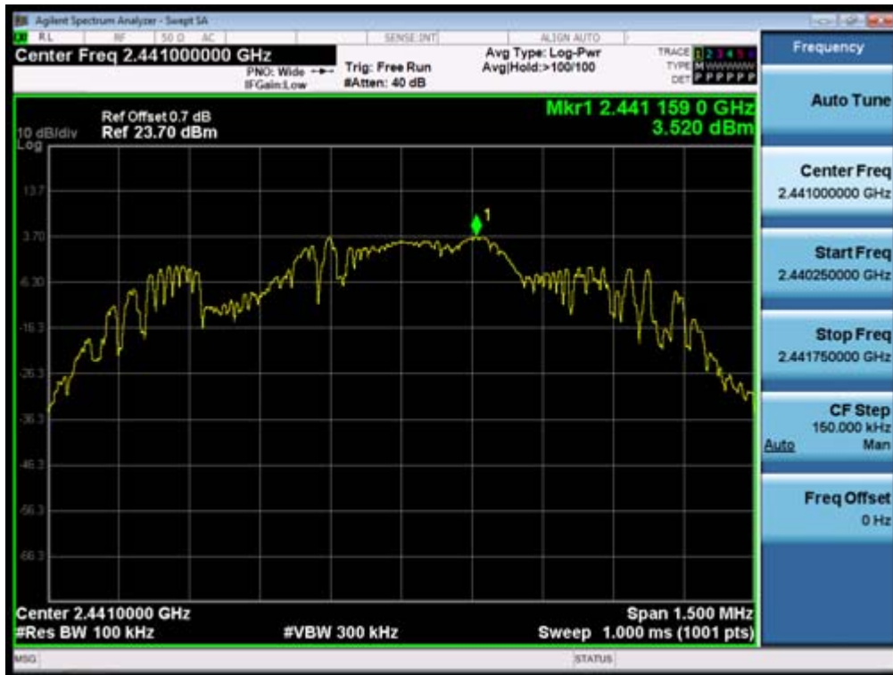
(Plot 4.9.3 B1: Channel 39: 2441MHz @ 8DPSK)
