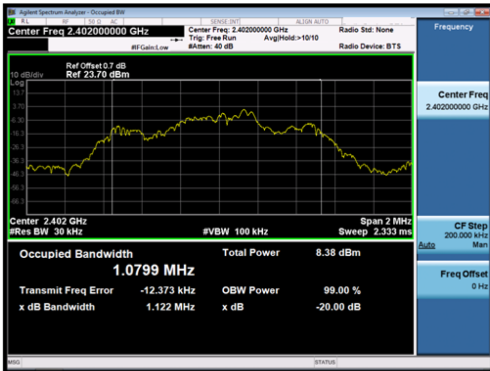
(Plot 4.4.2 A: Channel 00: 2402MHz @ 8DPSK)
