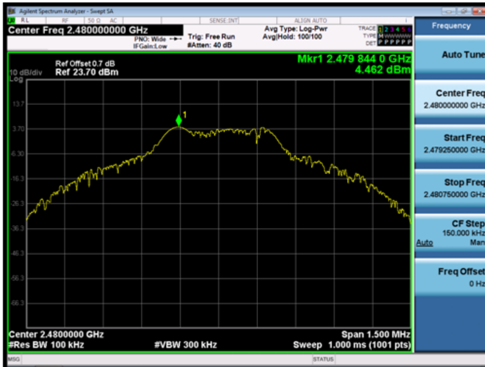
(Plot 4.9.1 C1: Channel 78: 2480MHz @ GFSK)
