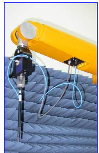
Figure 8. Probe setup on robot
