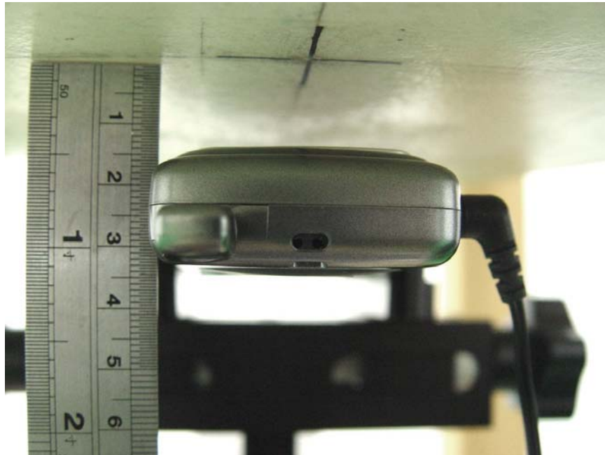
Fig. 9.7 Keypad Up With 1.5cm Gap
