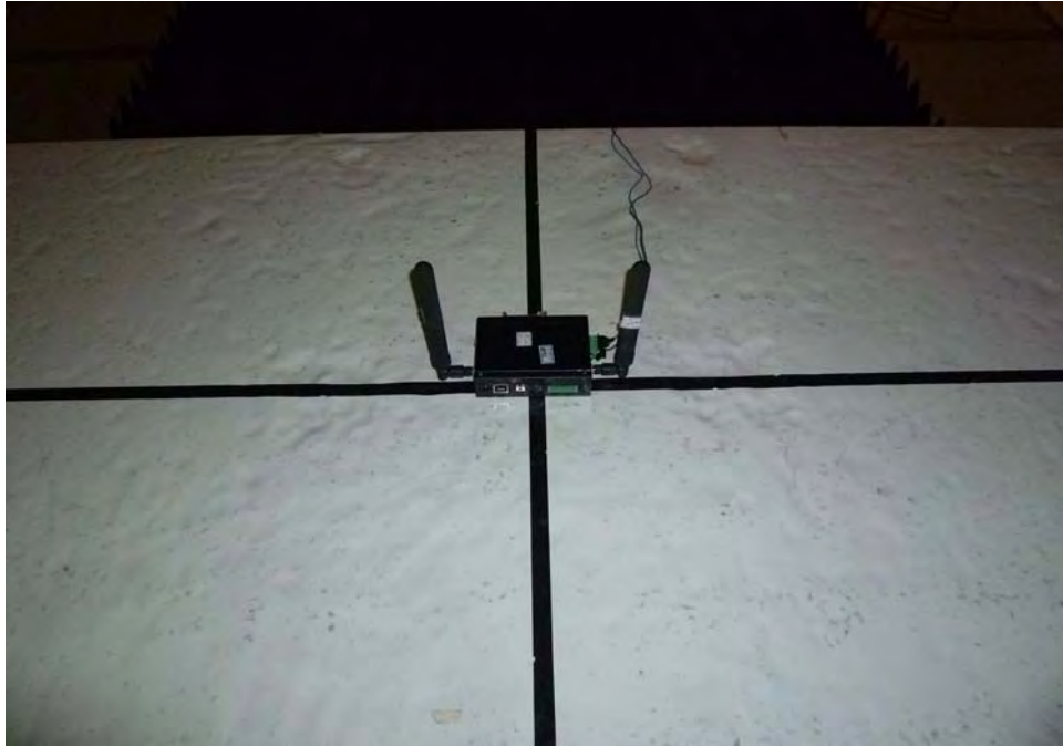
Description: Back View of Radiated Emission Test _ Above 1GHz
