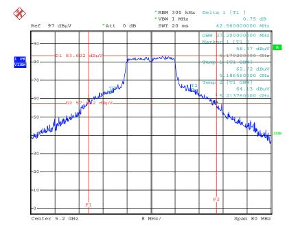
26dB Bandwidth and 99% Occupied Bandwidth Plot on Configuration IEEE 802.11a / Chain 1 + Chain 2 / 5200 MHz
