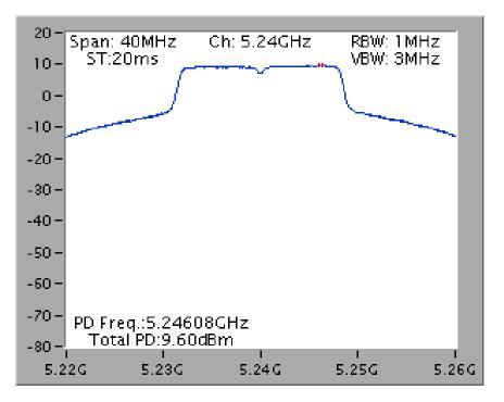
For Client mode (without radar detection function)
