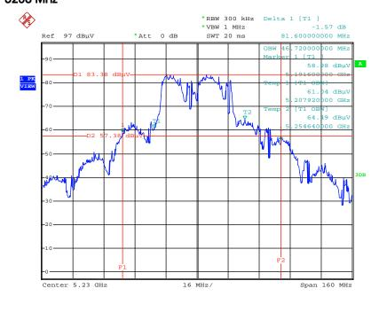
26dB Bandwidth and 99% Occupied Bandwidth Plot on Configuration IEEE 802.11n MCS8 HT40 / Chain 1 + Chain 2 / 5230 MHz
