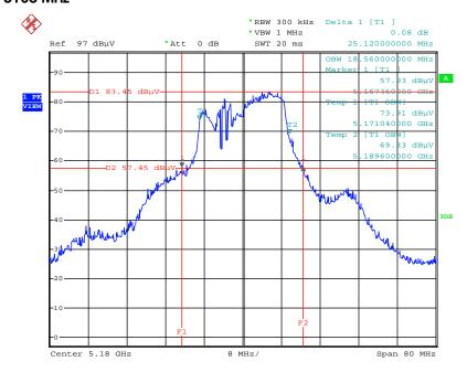
26dB Bandwidth and 99% Occupied Bandwidth Plot on Configuration IEEE 802.11n MCS8 HT20 / Chain 1 + Chain 2 / 5180 MHz
