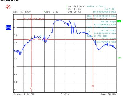
26dB Bandwidth and 99% Occupied Bandwidth Plot on Configuration IEEE 802.11n MCS8 HT20 / Chain 1 + Chain 2 / 5240 MHz
