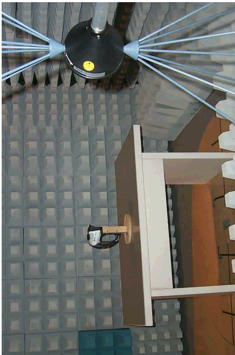
30764emi6.jpg Test set-up spurious emission (anechoic chamber)
