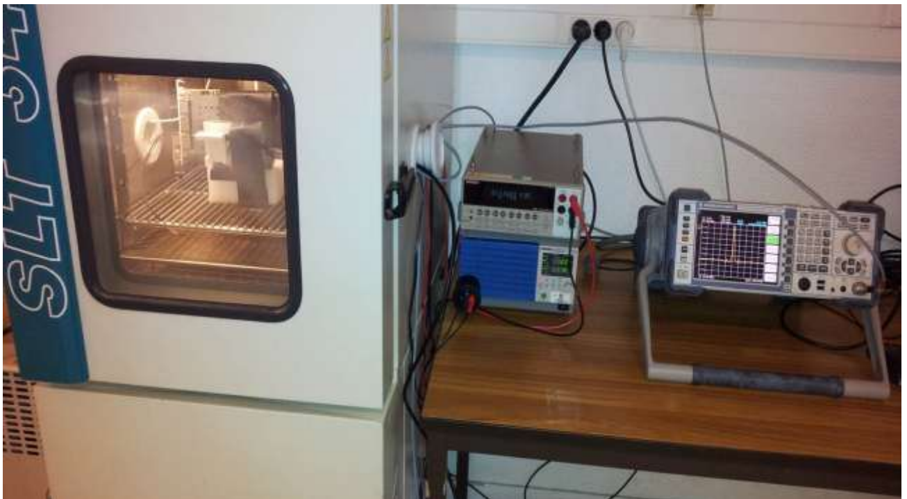
Test setup for frequency stability measurement in extreme conditions
