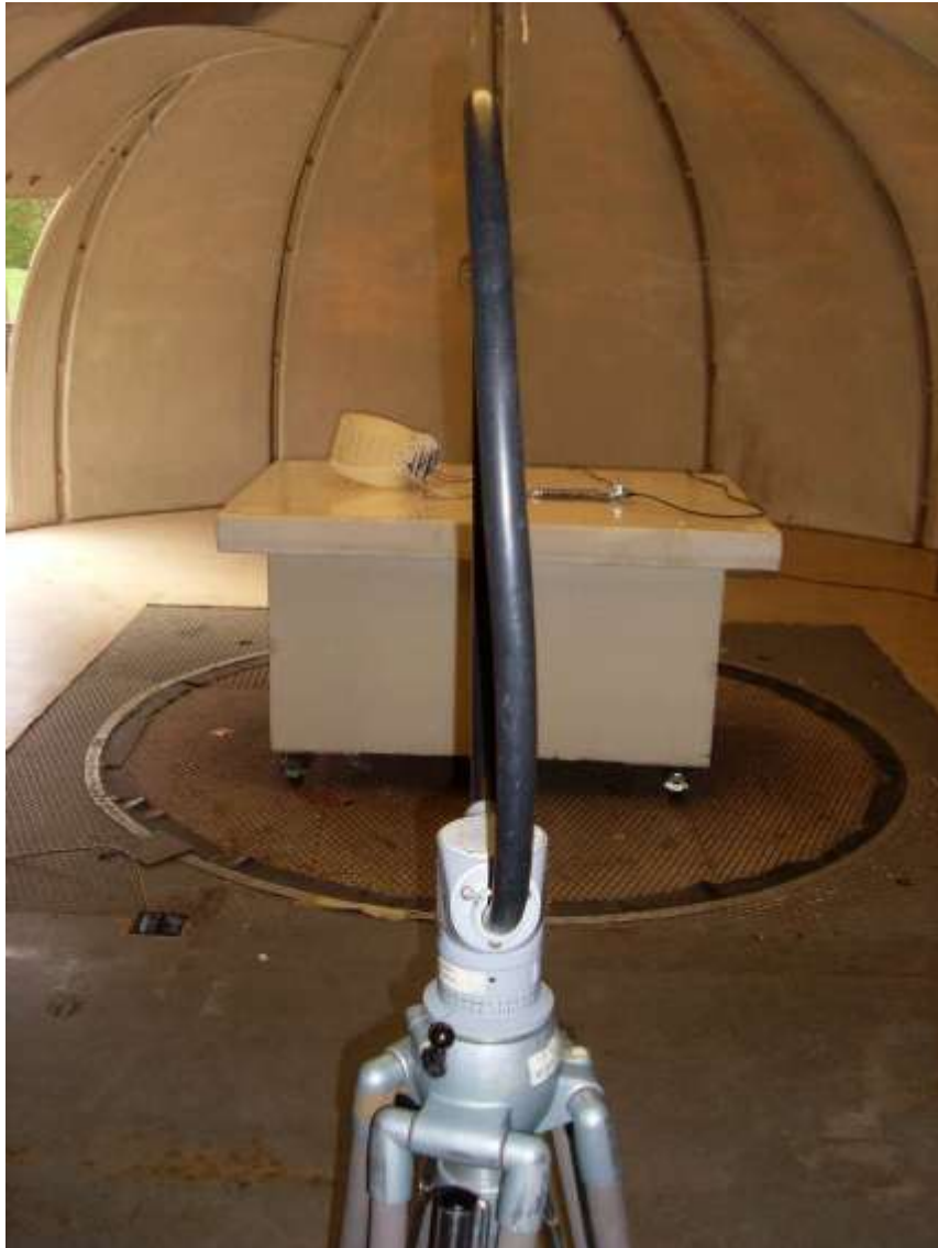
Test setup for radiated field strength
