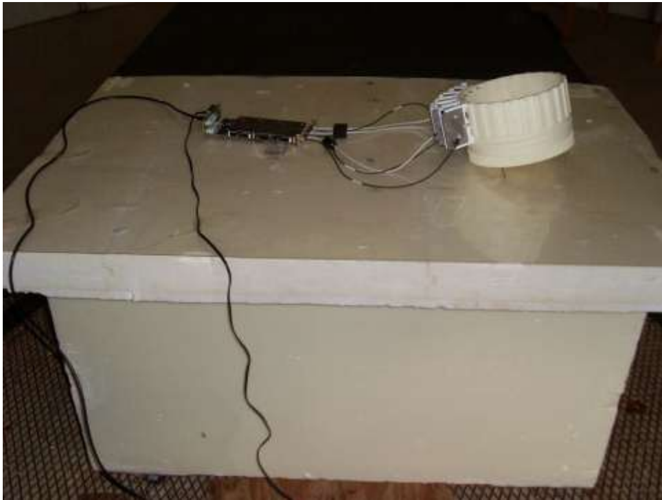
Test setup for radiated field strength
