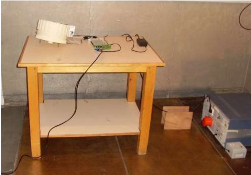
Test setup for power line conducted emissions
