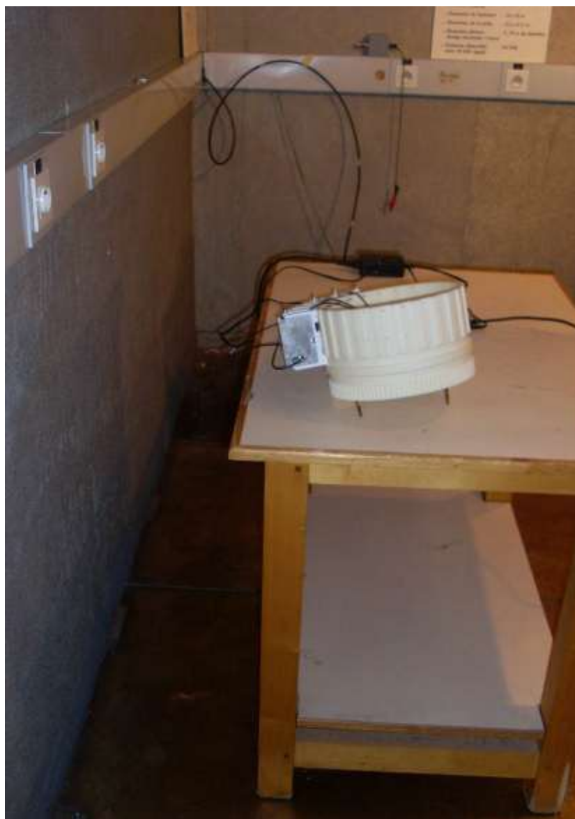
Test setup for power line conducted emissions
