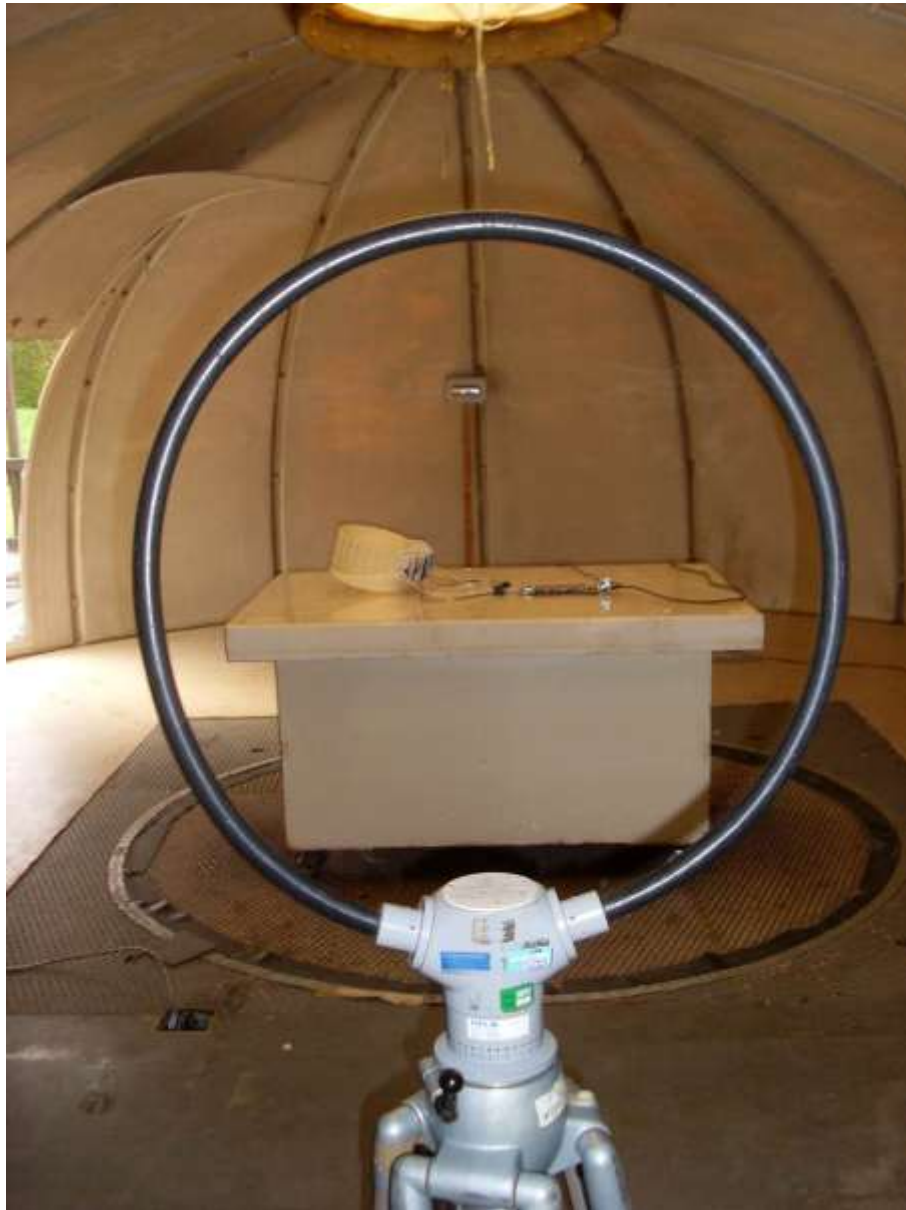
Test setup for radiated field strength
