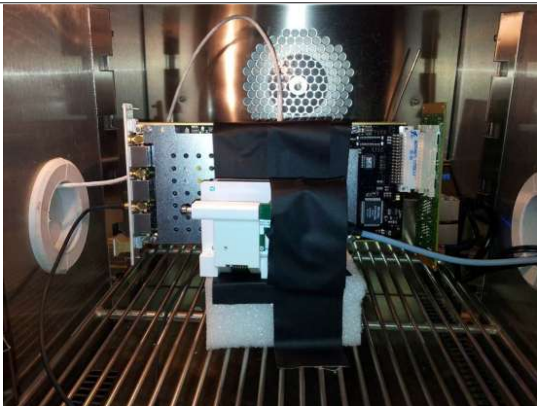
Photograph for Frequency tolerance
