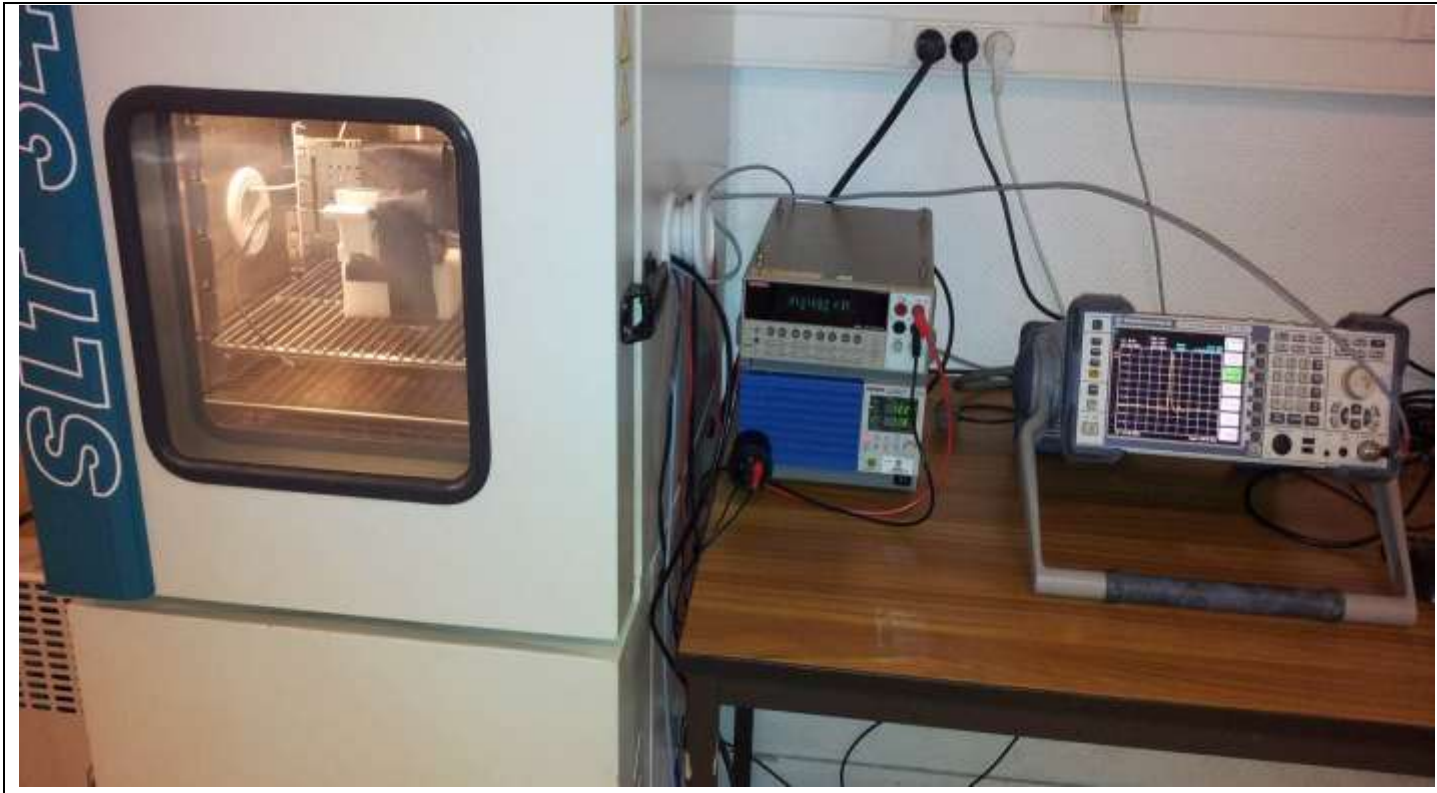
Photograph for Frequency tolerance
