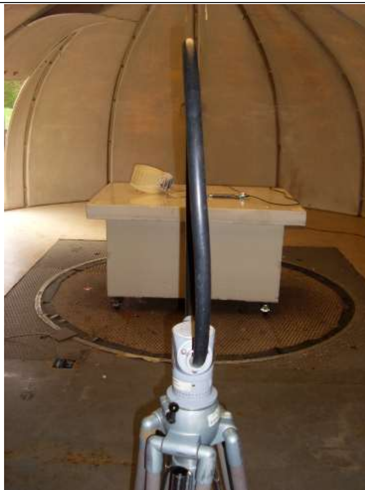
Photograph for Field strength below 30MHz
