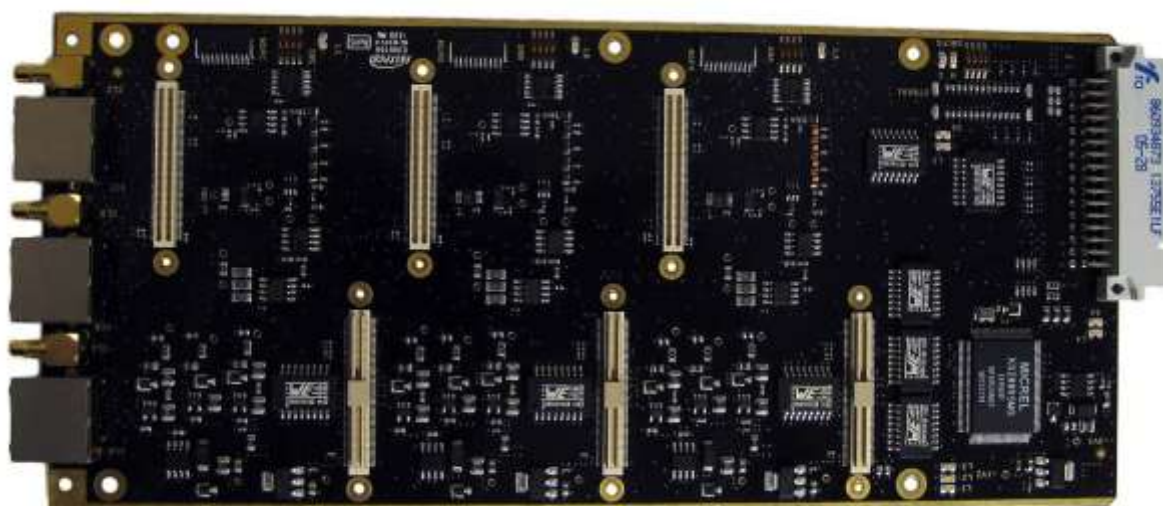
USN3e top view without US-nano daughterboards (RF)
