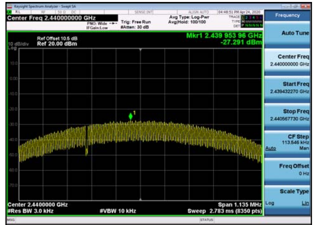
Power spectral density: 2440MHz
