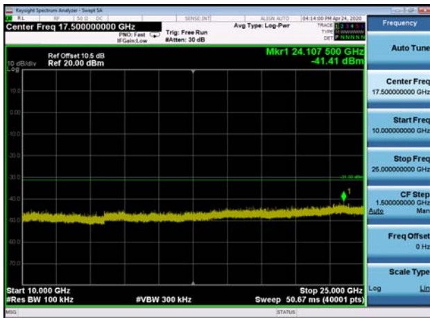
,Plot ,5Transmitter Spurious Emission : 2480,10000MHz~25000MHz
