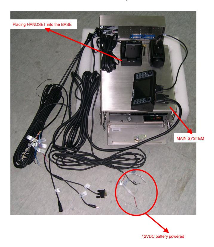
MAIN SYSTEM (Mobile Video System including VCR) is installed in the trunk of the cars.
